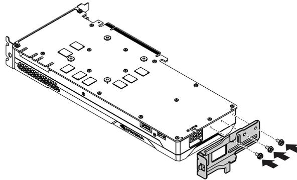
Figure 30. Installing a full-length PCIe card bracket
