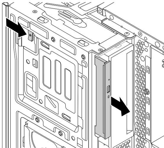
Figure 15. Removing the slim optical drive
