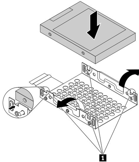
Figure 63. Installing the storage drive into the adapter
