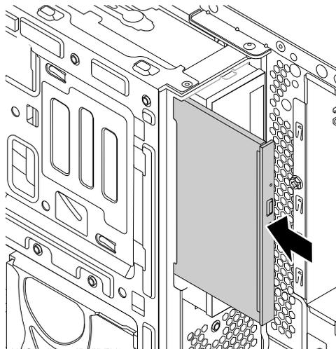
Figure 20. Installing the slim optical drive
