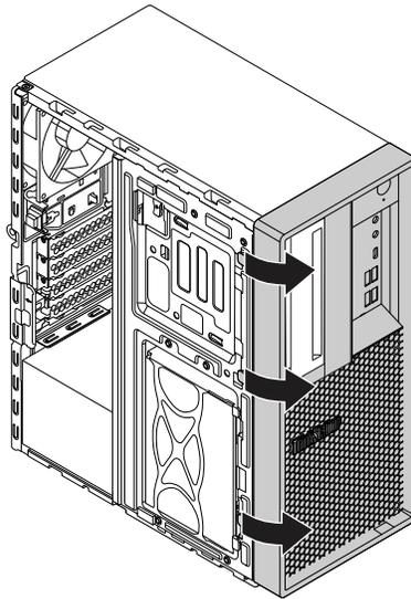
*Figure 13. Removing the front bezel*
