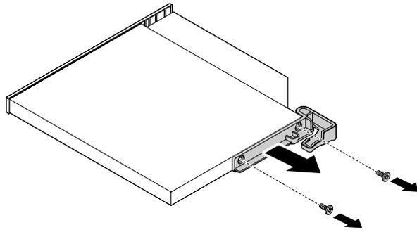
Figure 16. Removing the bracket
