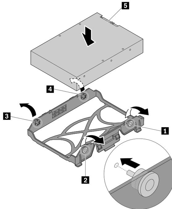
Figure 86. Installing the storage drive into the bracket
