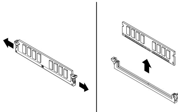
Figure 46. Removing a memory module
