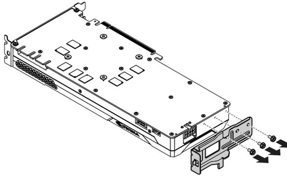
Figure 29. Removing a full-length PCIe card bracket
