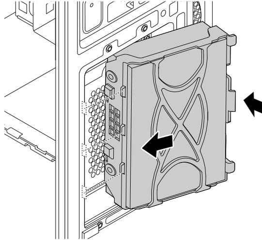
Figure 87. Installing the storage-drive
