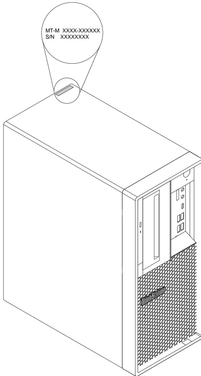
Figure 6. Machine type and model label
