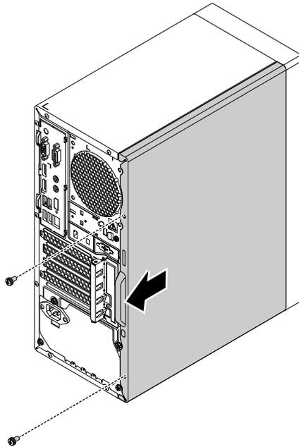
*Figure 12. Removing the computer cover*
