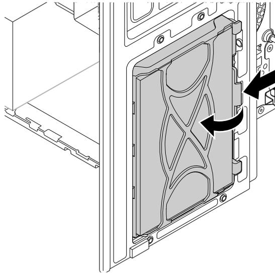
Figure 85. Removing the storage drive
