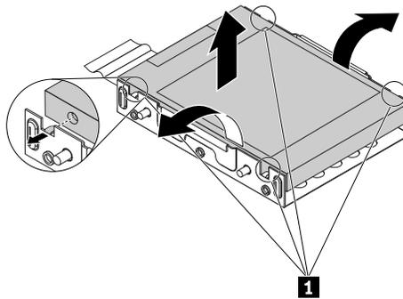
Figure 62. Removing the storage drive from the adapter
