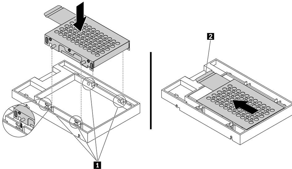
Figure 64. Installing the adapter into the converter
