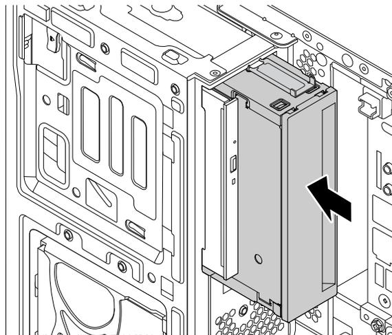
Figure 52. Installing the new flex storage enclosure
