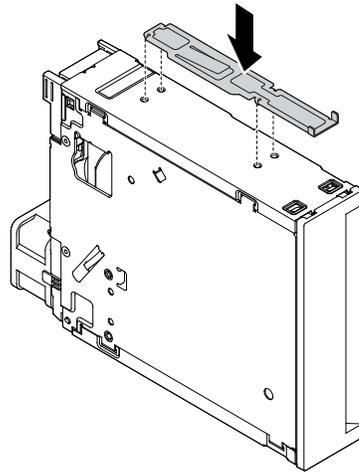
Figure 51. Installing the retainer
