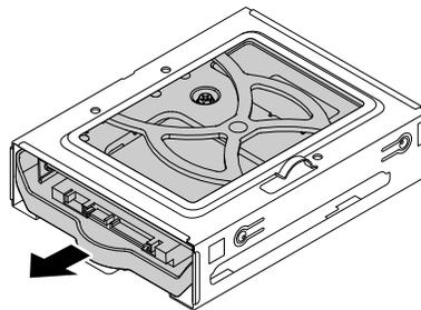
Figure 100. Removing the 2.5-inch storage drive
