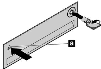
Figure 53. Opening the front-access storage enclosure cover
