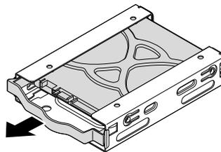
Figure 108. Removing the 2.5-inch storage drive
