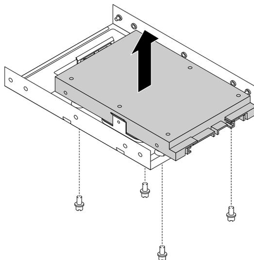
Figure 75. Removing the 2.5-inch storage drive from the storage-drive converter
