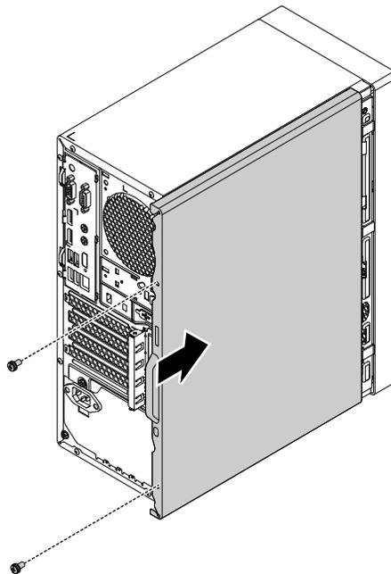
Figure 115. Reinstalling the computer cover
