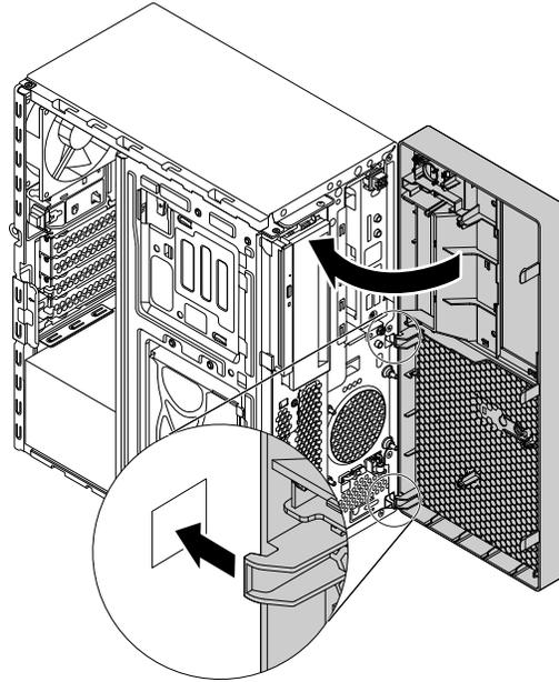
Figure 114. Reinstalling the front bezel
