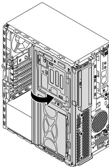
*Figure 14. Pivoting the drive bay assembly outward*
