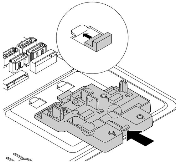
Figure 35. Installing the plastic holder
