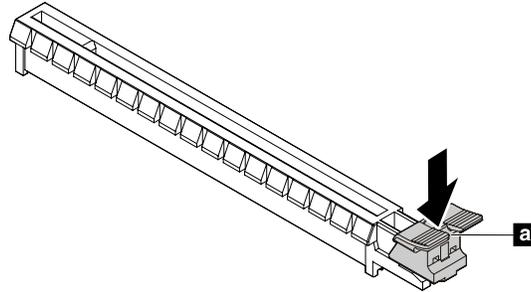
Figure 26. Disengaging the card retaining latch
