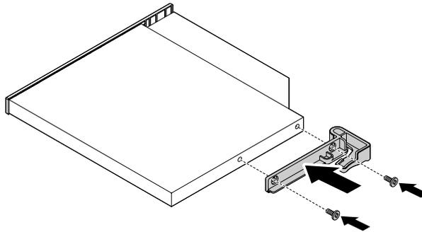
Figure 19. Installing the bracket
