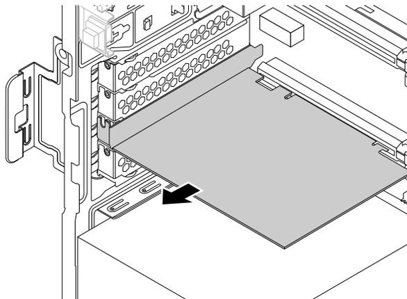
Figure 23. Removing a PCIe card
