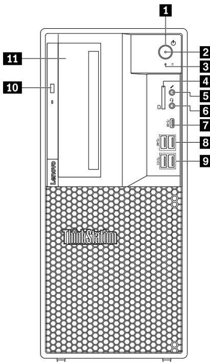
Figure 1. Front connectors, controls, and indicators
