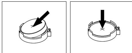
Figure 81. Installing the coin-cell battery
