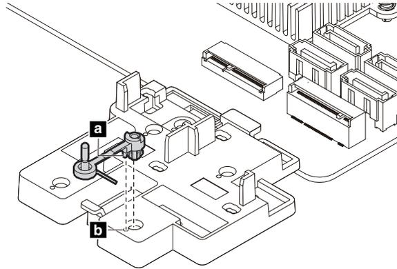
Figure 36. Installing the retention latch
