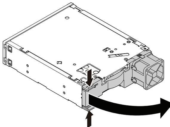
Figure 72. Opening the enclosure from the rear
