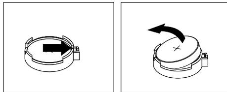
Figure 80. Removing the coin-cell battery
