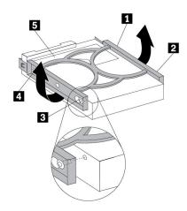
Figure 67. Installing the hard disk drive into the bracket
