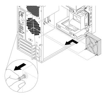
Figure 78. Installing the rear fan assembly
