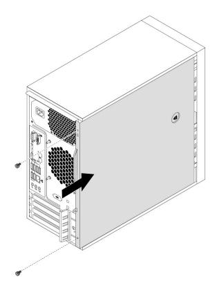
Figure 79. Reinstalling the computer cover
