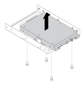
Figure 72. Removing the solid-state drive from the storage converter
