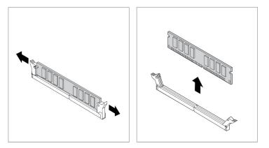
Figure 22. Removing a memory module
