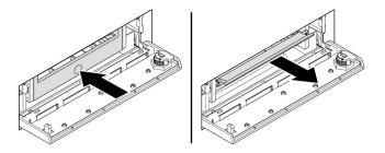
Figure 31. Removing the hard disk drive from the front-access storage enclosure
