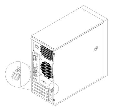
Figure 7. Installing a padlock
