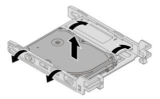
Figure 47. Flexing both sides of the bracket to remove the 2.5-inch internal storage drive
