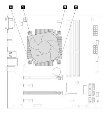
Figure 62. Removing the heat sink and fan assembly
