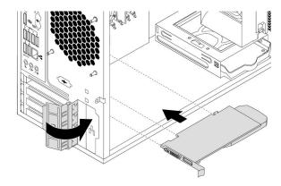
Figure 15. Installing a PCIe card
