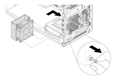
Figure 76. Installing the front fan assembly
