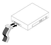
Figure 29. Connecting the cables to the rear of the new optical drive
