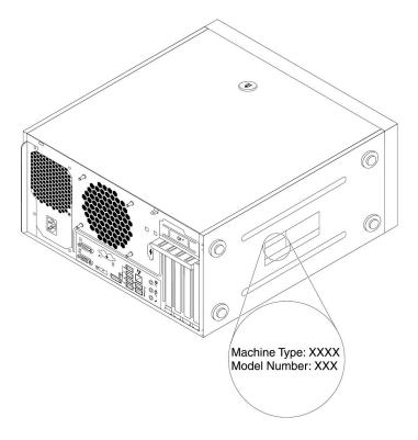
Figure 6. Machine type and model label
