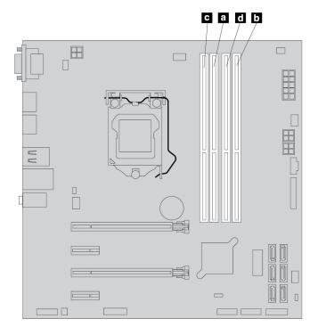
Figure 21. Memory module installation-order
