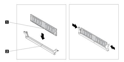
Figure 24. Installing a memory module
