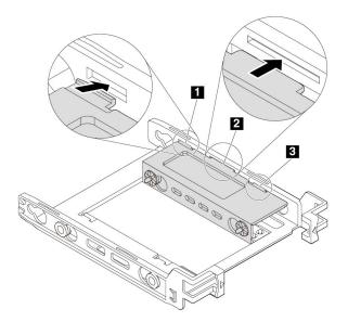
Figure 54. Inserting tabs 1 and 3 into the corresponding slots
