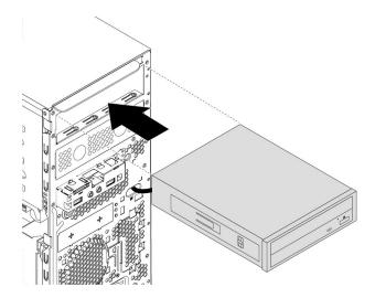
Figure 28. Installing the optical drive
