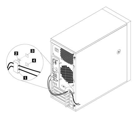
Figure 9. Installing a cable lock
