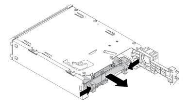
Figure 40. Removing the 3.5-inch internal storage drive from the rear
