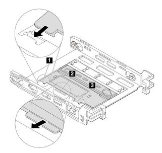
Figure 58. Inserting tabs 1 and 3 into the corresponding slots
