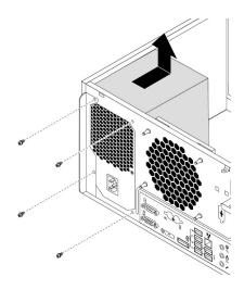
Figure 61. Removing the screws for the power supply assembly
