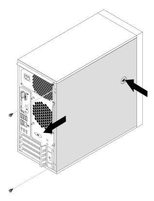
Figure 10. Removing the computer cover
