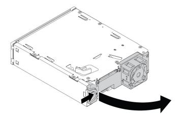
Figure 39. Opening the kit from the rear
