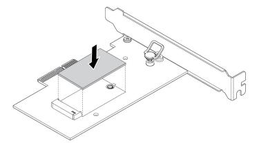
Figure 18. Installing the thermal pad
