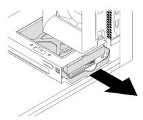
Figure 66. Removing the secondary hard disk drive
