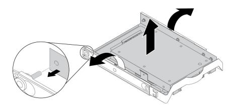
Figure 71. Removing the storage converter from the 3.5-inch storage drive bracket
