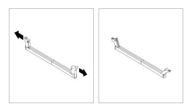
Figure 23. Opening the retaining clips
