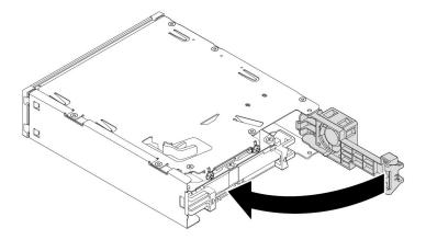
Figure 44. Pivoting the rear cover inward
