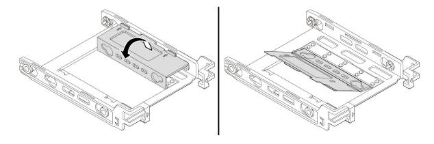
Figure 57. Unfolding the bracket
