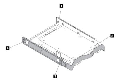
Figure 74. Installing the storage converter with the new solid-state drive into the storage drive bracket
