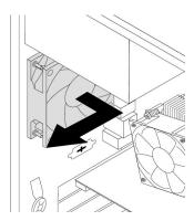
Figure 77. Removing the rear fan assembly
