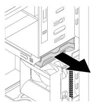
Figure 63. Removing the primary hard disk drive
