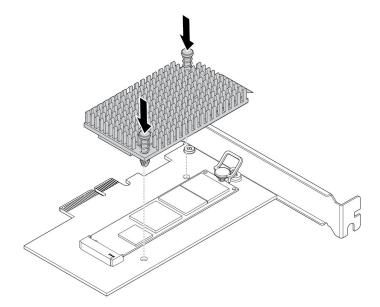
Figure 20. Installing the heat sink
