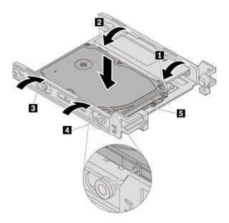
Figure 48. Installing the new 2.5-inch internal storage drive into the bracket
