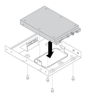
Figure 73. Installing the new solid-state drive into the storage converter
