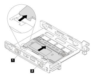
Figure 52. Pivoting the bracket
