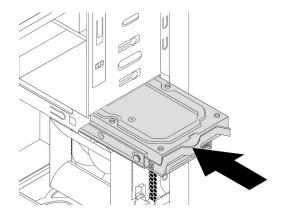
Figure 65. Installing the primary hard disk drive
