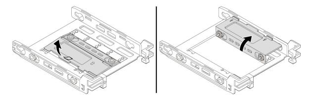
Figure 53. Folding the bracket
