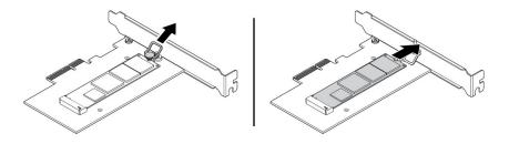
Figure 17. Removing the M.2 solid-state drive
