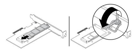
Figure 19. Installing the M.2 solid-state drive
