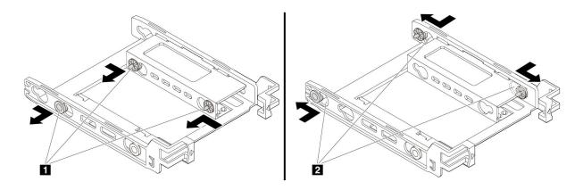
Figure 55. Removing three pins 1 and installing them into slots 2
