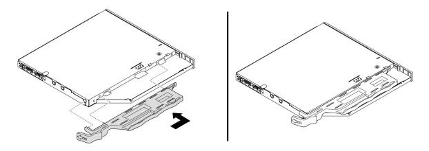
Figure 37. Installing the bracket to the new slim optical drive
