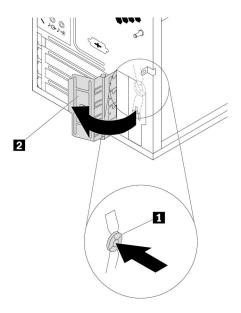
Figure 12. Opening the PCIe card latch
