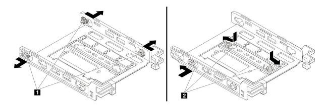
Figure 51. Removing three pins and installing them into new slots
