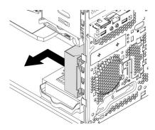
Figure 75. Removing the front fan assembly
