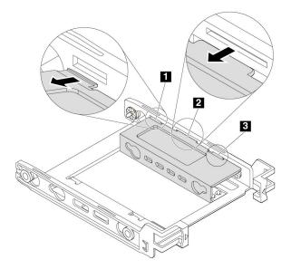
Figure 56. Releasing tabs 1, 2, and 3 from the corresponding slots
