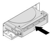
Figure 34. Installing the hard-disk-drive bracket
