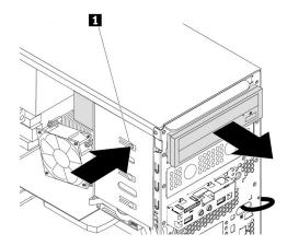
Figure 26. Removing the optical drive
