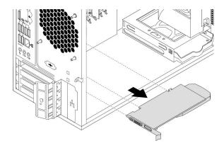
Figure 13. Removing a PCIe card
