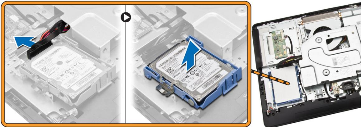
6. Pry the hard-drive bracket apart to release the hard drive. Remove the hard drive from the hard-drive bracket.
