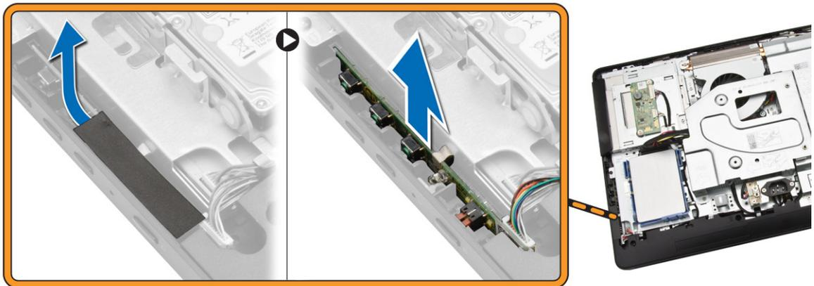
4. Disconnect the power-switch cable from the power-switch board to remove it from the computer.
