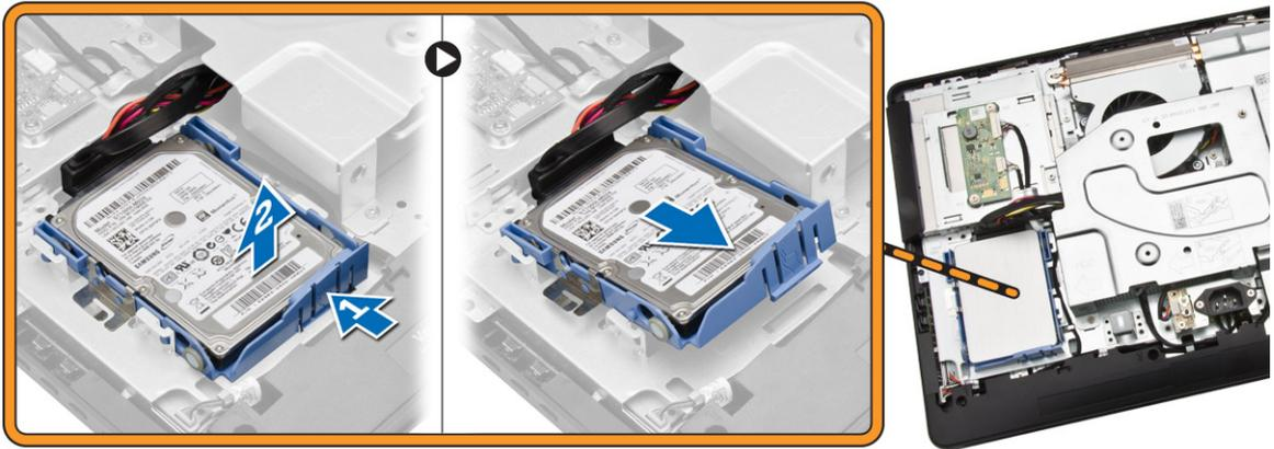
4. Slide and remove it to access the hard-drive cable.
