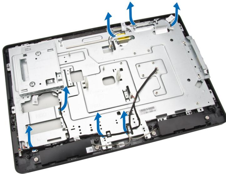
4. Remove the screws that secure the display bracket to the computer. Lift and remove the display bracket from the computer.
