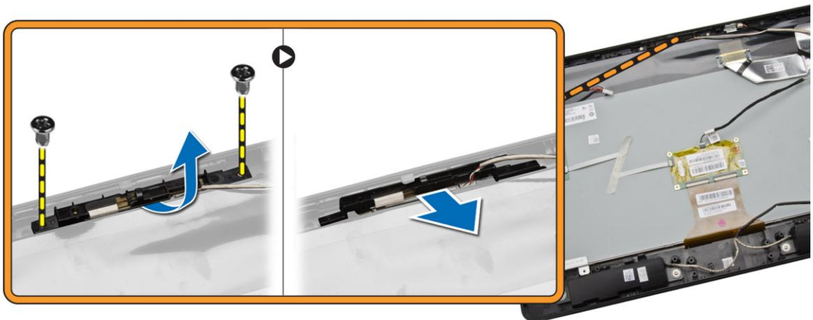
4. Disconnect the camera cable from the camera and remove the camera from the computer.
