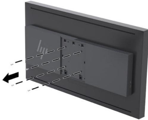
2. Install the included back plate cover over the mounting screws on the rear of the display.
