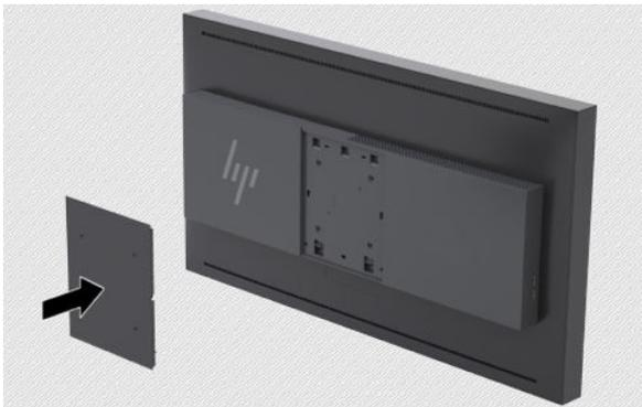
3. To mount the display head directly to a mounting fixture, use the four screws removed from the VESA holes on rear of the display head and install them to attach the mounting device to the rear of the display.
