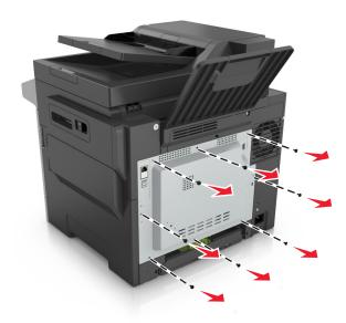
3 Slightly open the controller board access cover, and then shift to the right to remove it.
