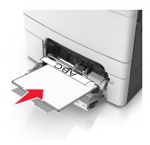
• Load envelopes with the flap side up and against the right side of the paper guide.
