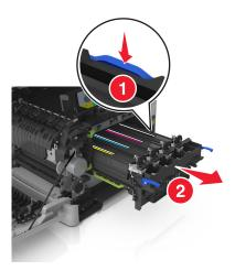
**8** Remove the used developer unit.
