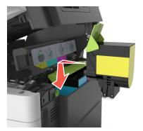
**5** Slide and hold the release latch on the right side of the printer, and then slowly close the top door.
