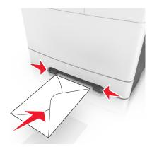
2 Feed paper into the manual feeder only to the point where its leading edge can contact the paper guides.
