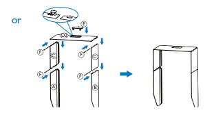
3. Slide down the shading hood on the top of the monitor.
