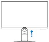
2. Place the monitor face down on a smooth surface. Pay attention not to scratch or damage the screen. Then lift the monitor stand.
