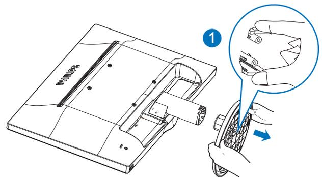
3. Press the release button to detach the base column.
