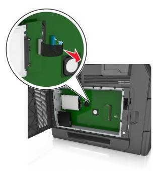
**3** Remove the screws holding the printer hard disk in place.
