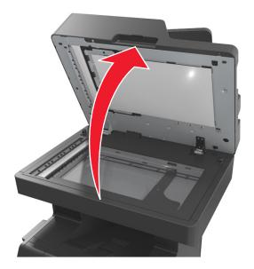
If the jam is in the bottom ADF door or ADF exit bin, then open the bottom ADF door, and then firmly grasp the jammed paper on each side.
