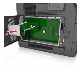
**c** Insert the plug of the printer hard disk interface cable into the receptacle of the ISP.
