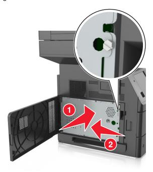
Tighten the screws on the shield.
