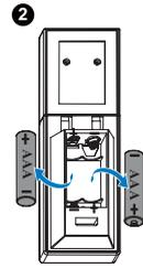
3 Insert the batteries and align their polarity correctly according to the marking in the battery compartment.
