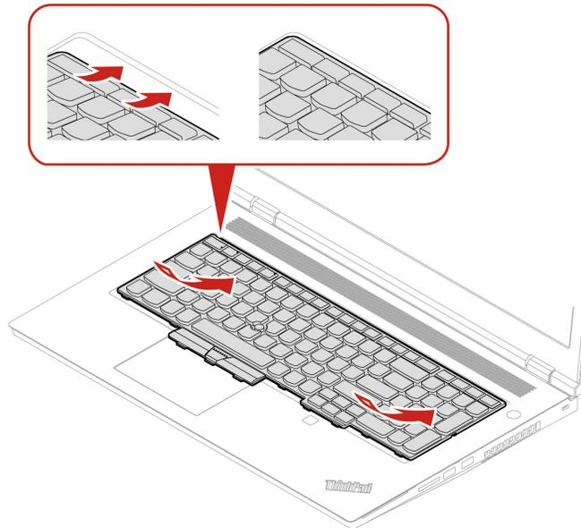
10. Slide the keyboard in the direction as shown. Ensure that the latches are secured under the keyboard frame.
