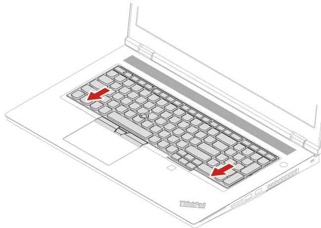
11. Turn over the computer and tighten the screws to secure the keyboard.
