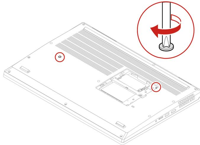
12. Reinstall the bottom door. Then, turn over the computer.
