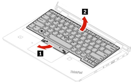
8. Put the keyboard on the palm rest as shown and detach the connectors. Then remove the keyboard.
