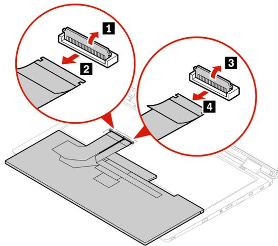
9. Attach the connectors and turn the keyboard over as shown.
