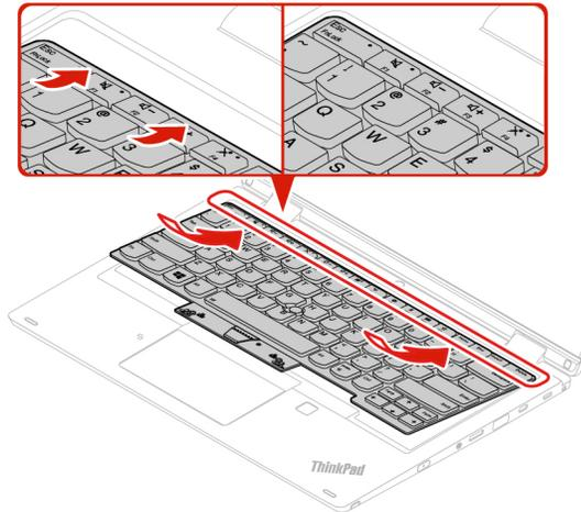
11. Slide the keyboard in the direction as shown by the arrows. Ensure that the latches are secured under the keyboard frame.
