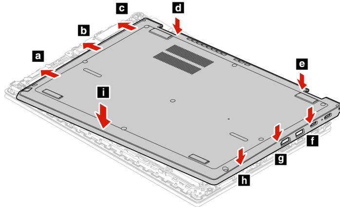
7. Ensure that the latches of the base cover assembly are secured in place and then tighten the screws.
