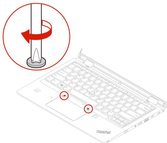
13. Take the new TrackPoint buttons out of the new keyboard package. Install the TrackPoint buttons as shown.
