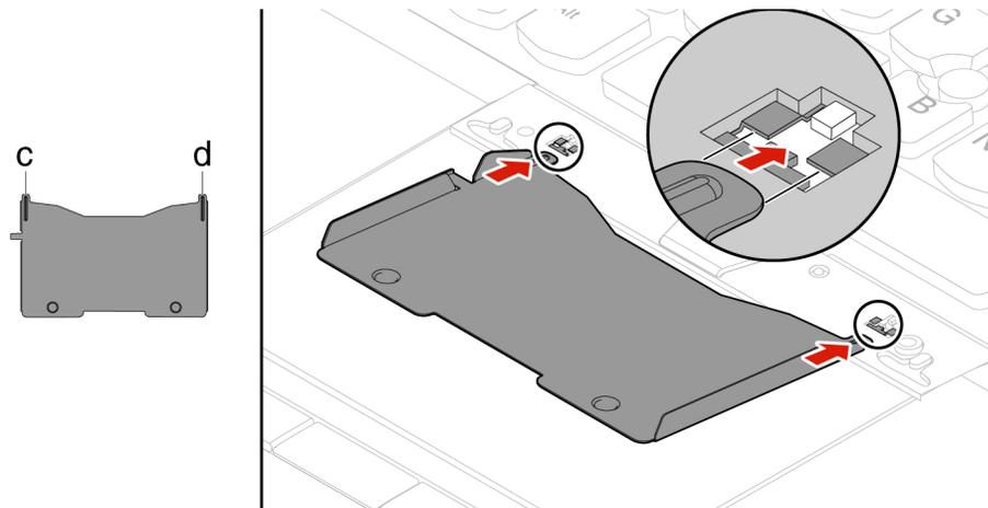
6. Pivot the tool in the direction as shown to release the keyboard **1**. Push the keyboard in the direction as shown by arrows **2** to release the latches from the keyboard bezel.
