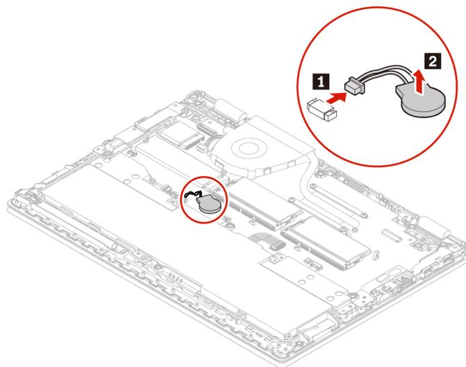
6. Install the new coin-cell battery **1**, and then attach the connector **2**.
