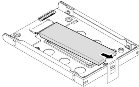
To install the new M.2 solid-state drive in the internal-storage-drive bay, do the following:
