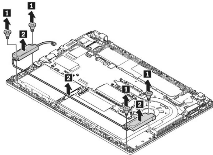
8. Install the new speaker assembly in place **1** and route the speaker cables. Then install the screws to secure the speaker assembly **2**.
