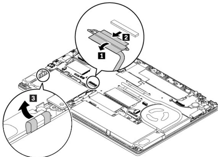
7. Remove the 2.5-inch internal storage drive by pulling the tape.
