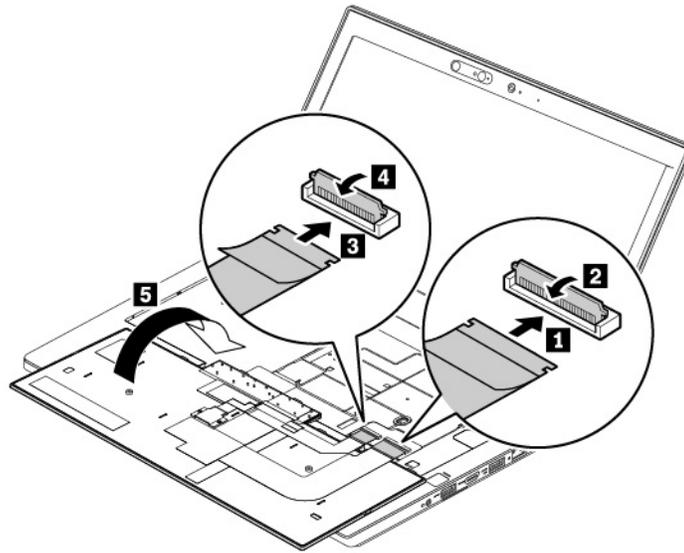
2. Insert the keyboard into the keyboard bezel as shown. Ensure that the top edge of the keyboard (the edge that is close to the computer display) is under the frame of the keyboard bezel.
