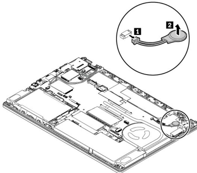
7. Install the new coin-cell battery **1** and attach the connector **2**.
