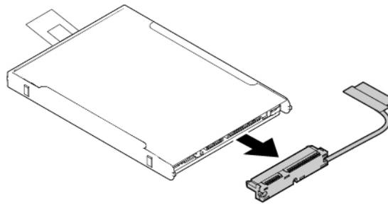
9. Detach the bracket from the 2.5-inch internal storage drive.
