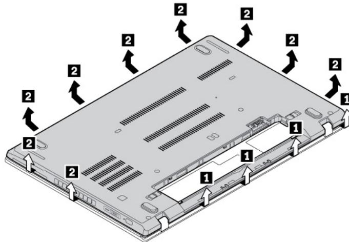
9. Install the new base cover assembly in place **1**. Ensure that the latches of the base cover assembly are secured under the base cover assembly. Then tighten the screws to secure the base cover assembly **2**.
