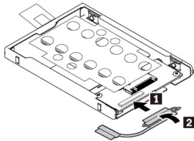
5. Insert the adapter **1** and then pivot it downward **2**. Ensure that the adapter is seated in place.
