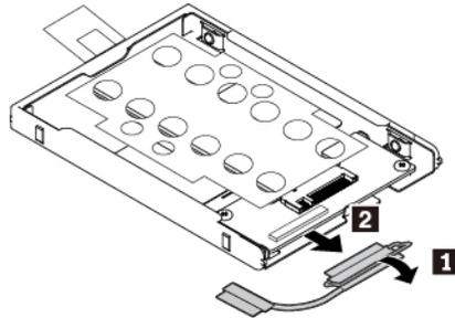
9. Remove the two screws that secure the protective cover **1**, and then remove the cover **2**.
