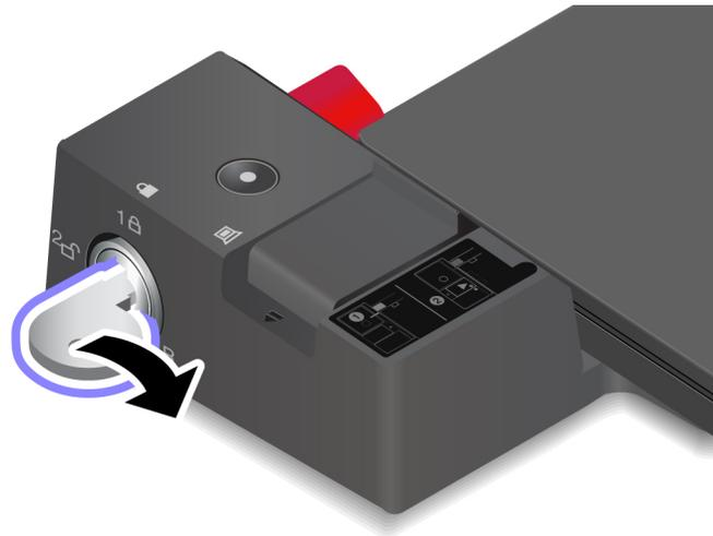
**Attention:** When the computer is attached to a docking station, do not pick up the assembly by taking hold of the computer only. Always hold the whole assembly. Otherwise the docking station might drop down.
