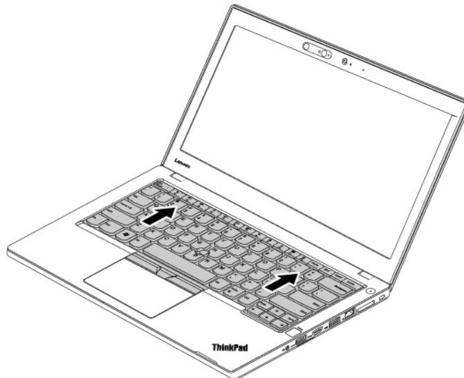
7. Pivot the keyboard slightly upward as shown by arrow **1**. Then turn over the keyboard as shown by arrow **2**.
