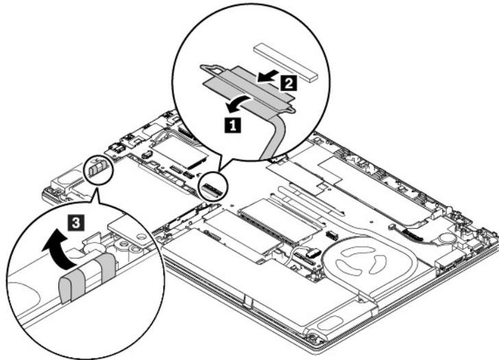
7. Remove the M.2 solid-state-drive adapter by pulling the tape.
