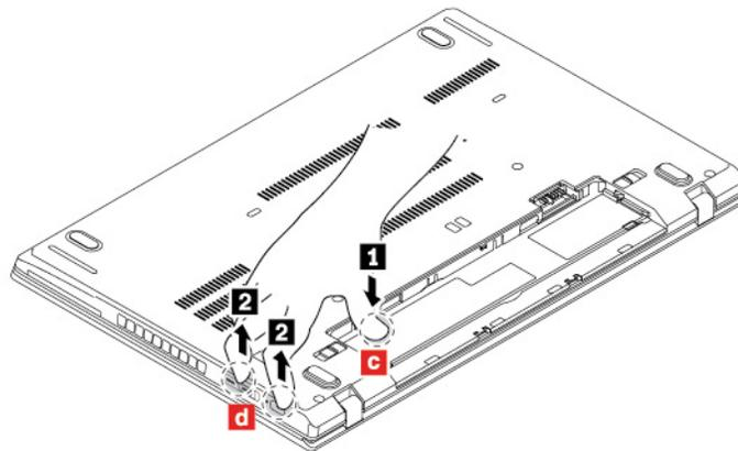
8. Remove the base cover assembly in the numeric order as shown.
