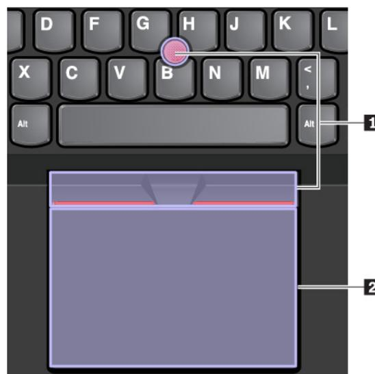
By default, both the TrackPoint pointing device and the trackpad are active with the touch gestures enabled. To change the settings, see “Customizing the ThinkPad pointing device” on page 23.
