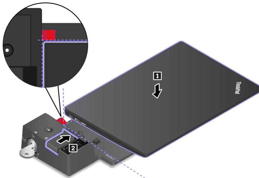
5. Check the docking status indicator. The docking status indicator turns on when the computer is successfully docked.
