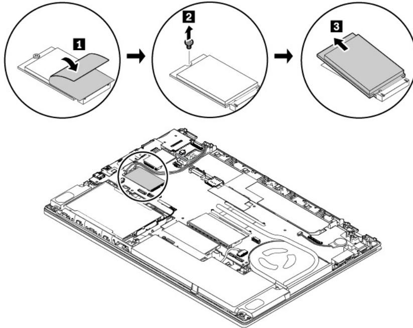
7. Install the new M.2 solid-state drive by doing the following:
