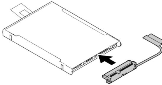
3. Insert the new internal storage drive **1** and then pivot it downward **2**. Ensure that the new internal storage drive is seated in place.
