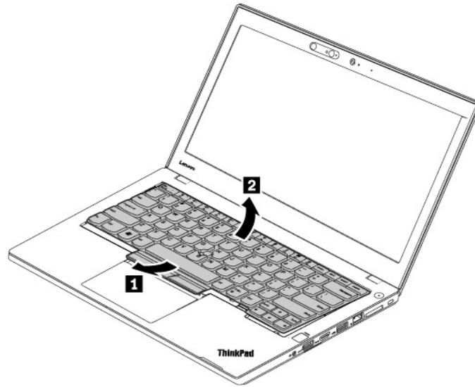
8. Put the keyboard on the palm rest and detach the connectors. Then remove the keyboard.
