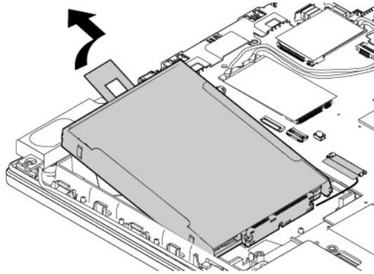
8. Disconnect the cable from the 2.5-inch internal storage drive.
