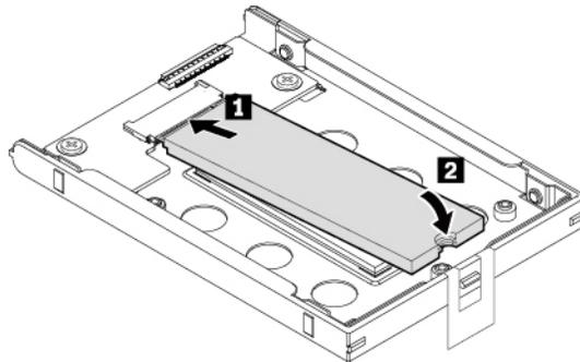
2. Install the screw to secure the M.2 solid-state drive.
