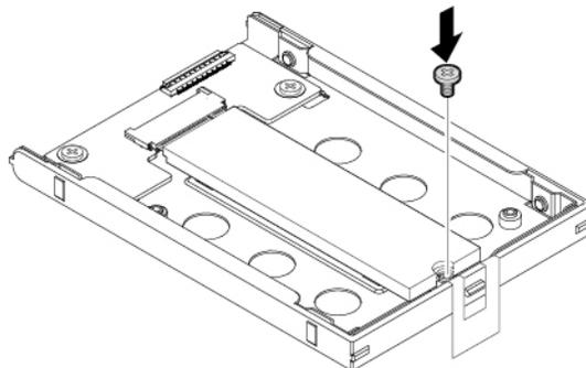
3. Install the protective cover and then install the two screws to secure the cover.
