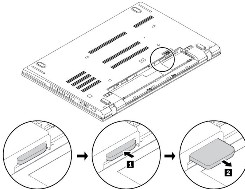
6. Note the orientation of the new nano-SIM card and then insert it into the slot completely until it clicks into position.
