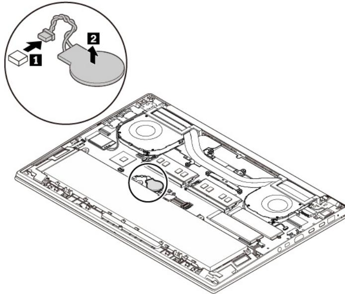
6. Install the new coin-cell battery and attach the connector.
