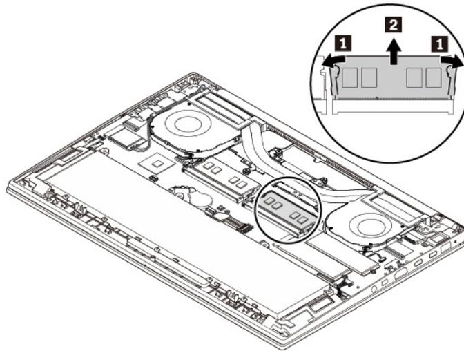
6. Insert the new memory module into the memory slot at an angle of about 20 degrees **1**. Pivot the memory module downward until it snaps into place **2**. Ensure that the memory module is firmly installed in the memory slot and cannot be moved easily.
