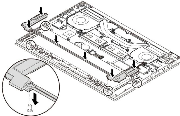
8. Route the cables as shown and attach the connector of the speaker assembly.
