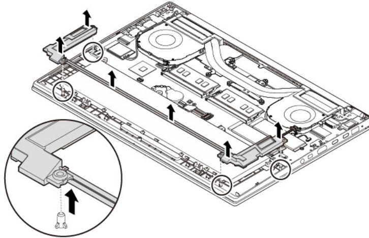
7. Install the new speaker assembly in place.
