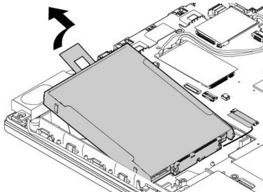
8. If you also want to replace the M.2 solid-state-drive cable, disconnect the cable from the M.2 solid-state-drive converter.
