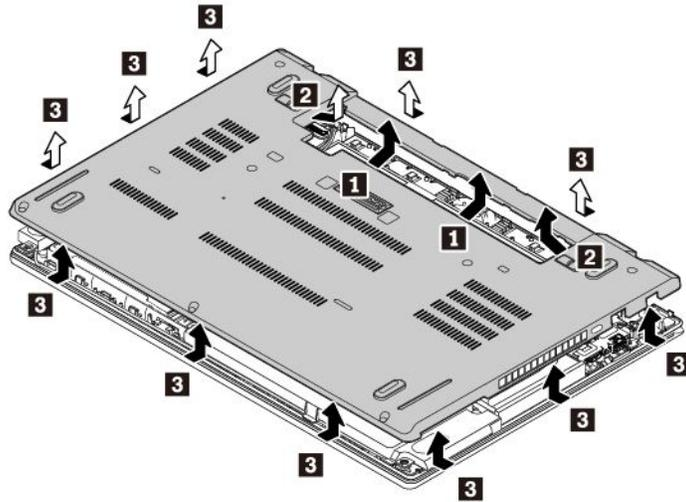
7. Install the new base cover assembly in place **1**. Ensure that the latches of the base cover assembly are secured under the base cover assembly. Then tighten the screws to secure the base cover assembly **2**.
