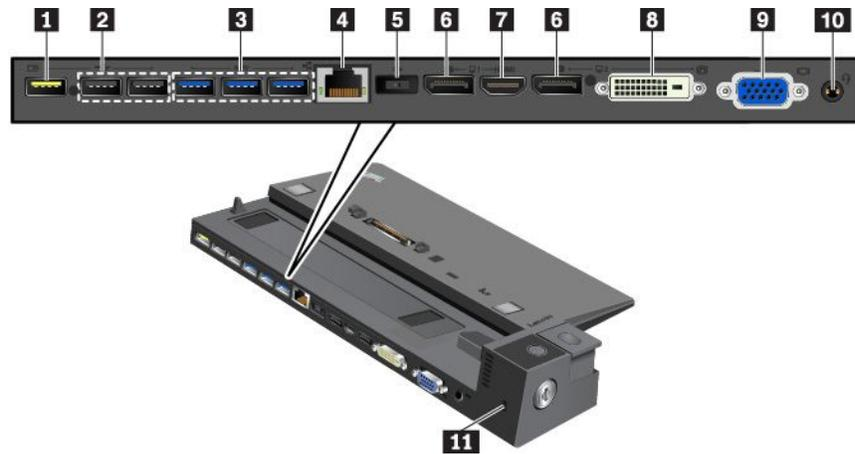
**1 Always On USB 2.0 connector:** Connect USB-compatible devices or charge some mobile digital devices and smartphones.
