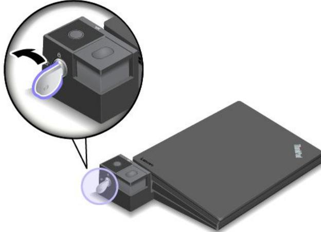
3. Press the eject button to eject the computer **1**, and then grasp both sides of the computer to remove it **2**.
