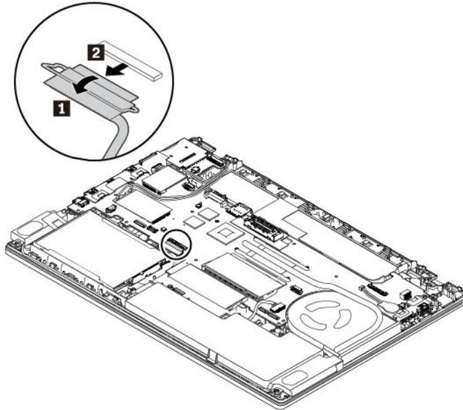
7. Pull the tape to remove the 2.5-inch storage drive and its bracket.
