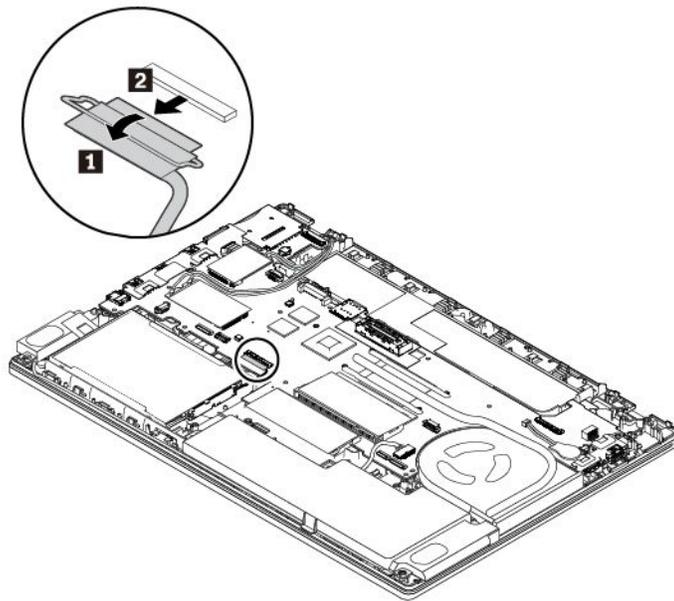
7. Pull the tape to remove the M.2 solid-state-drive converter and its bracket.
