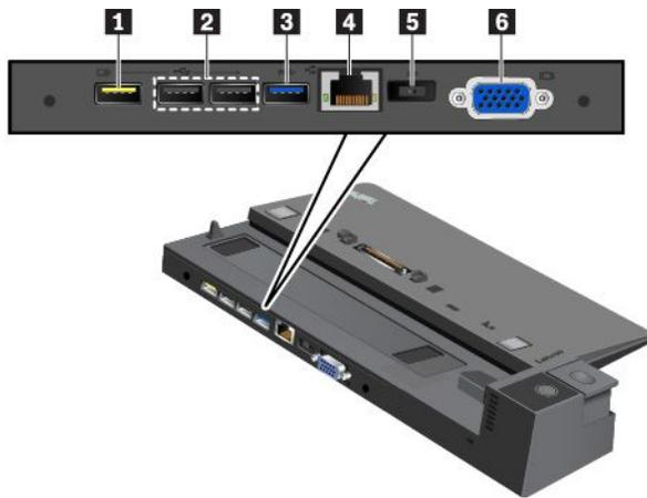
**1 Always On USB 2.0 connector:** Connect USB-compatible devices or charge some mobile digital devices and smartphones.
