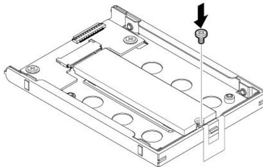
3. Install the M.2 solid-state-drive adapter and then install the two screws to secure the M.2 solid-state-drive adapter.
