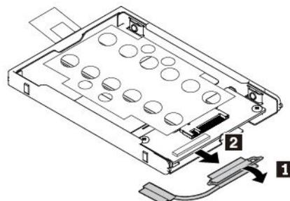
9. Remove the two screws that secure the M.2 solid-state-drive adapter **1**, and then remove the adapter **2**.
