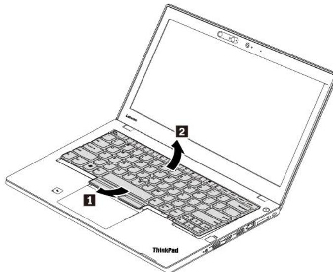
9. Put the keyboard on the palm rest and detach the connectors. Then remove the keyboard.
