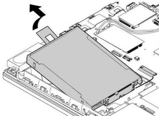
8. Disconnect the cable from the 2.5-inch storage drive.
