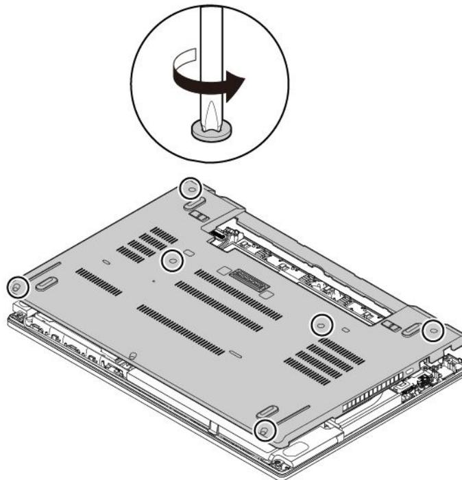
6. Remove the base cover assembly in the numeric order as shown.
