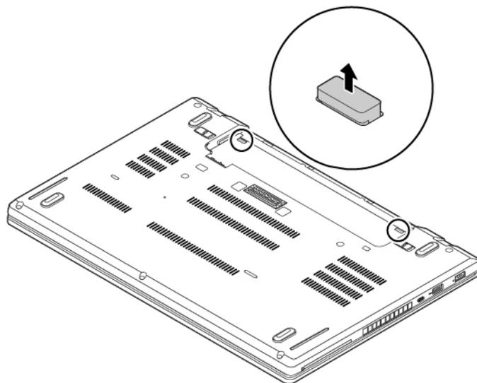
7. Turn the computer over and open the display. Push hard in the direction as shown to release the latches from the keyboard bezel.
