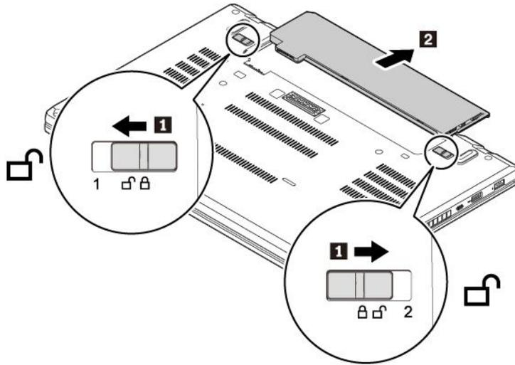
5. Insert a new battery until it clicks into place. Ensure that the latches are in the locked positions.
