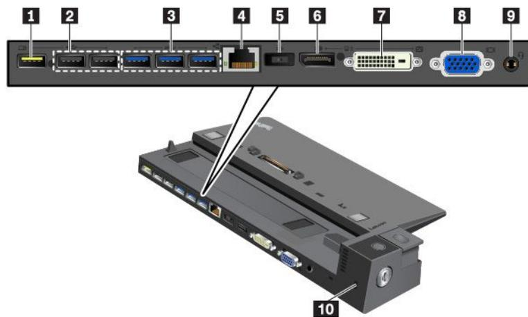
**1 Always On USB 2.0 connector:** Connect USB-compatible devices or charge some mobile digital devices and smartphones.
