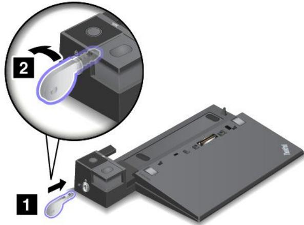
2. Attach your computer to the docking station as shown until you hear a click **1**. Turn the system lock key to the locked position (vertical) **2**.
