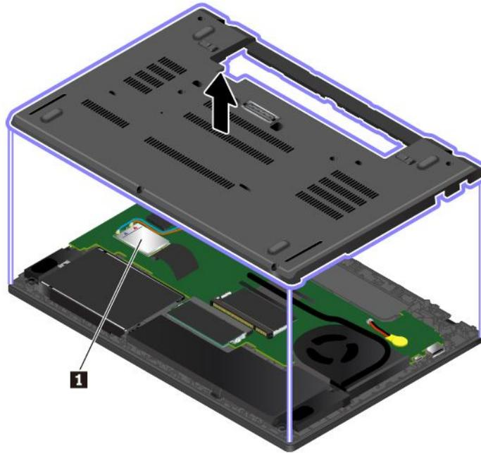
**Note:** For the user-installable wireless module, ensure that you use only a Lenovo-authorized wireless module for the computer. Otherwise, an error message will be displayed and the computer will beep when you turn on the computer.
