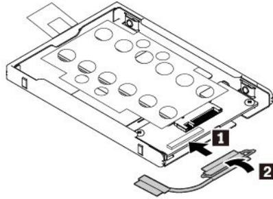
5. Insert the converter **1** and then pivot it downward **2**. Ensure that the converter is seated in place and the tape does not cover the speaker.
