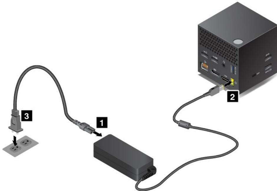
1. Connect the power cord to the ac power adapter.
