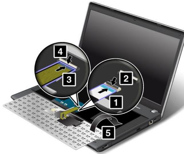
2. Insert the keyboard into the space under the frame of the keyboard bezel as shown.
