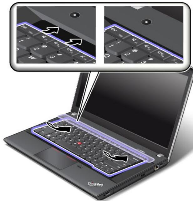
3. Reveal the screw heads by sliding the keyboard frame forward with the keyboard multi-tool. Ensure that the screw heads are exposed completely.
