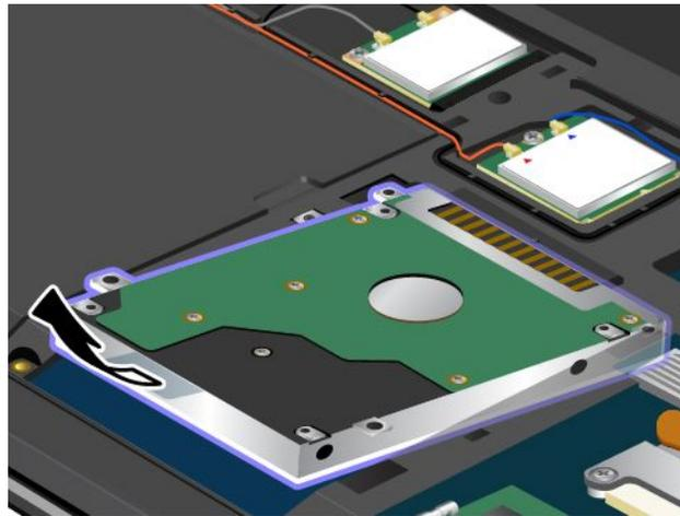
7. Place the new hard disk drive or solid-state drive into the drive bay.
