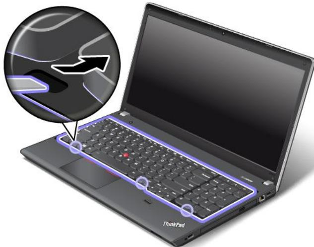
7. Loosen the screws that secure the keyboard with the keyboard multi-tool.
