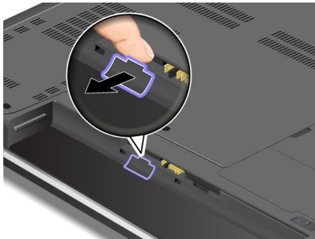
6. To reveal the screw heads beneath the keyboard frame, slide the keyboard frame forward by 2.5 mm (0.1 inch) with the keyboard multi-tool.
