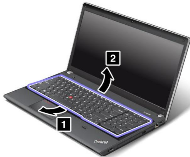
9. Gently put the keyboard on the palm rest and detach the connectors. Then remove the keyboard.
