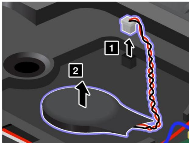
6. Install the backup battery **1**. Then attach the connector **2**.
