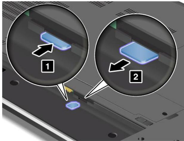
5. Hold the new card with the metal contact facing upward and going into the slot first. Then, insert the card firmly into the slot until you hear a click.
