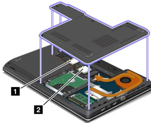
To remove the wireless LAN card for repair or replacement, see “Replacing a wireless LAN card” on page 92.
