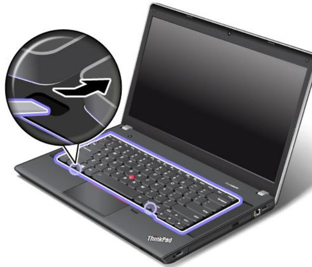
4. Tighten the screws with the keyboard multi-tool to secure the keyboard in place.
