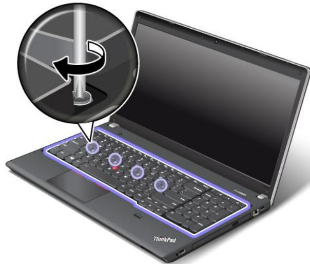
5. Slide the keyboard frame backward by 2.5 mm (0.1 inch) with the keyboard multi-tool. Hide the latches of the keyboard frame under the keyboard bezel by pushing the latches with your finger as shown.
