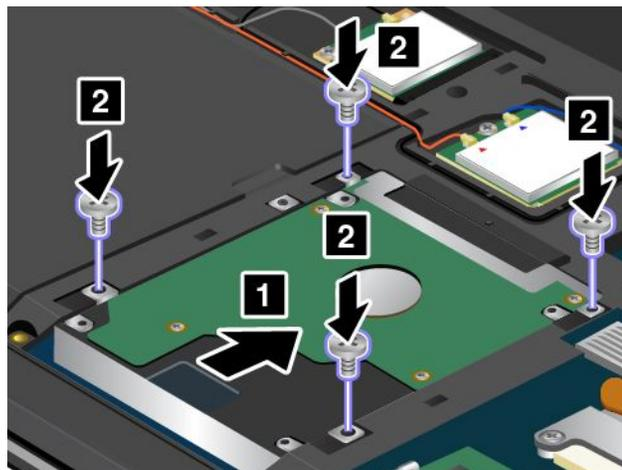
9. Reinstall the computer cover **1**. Then tighten the screws **2**.
