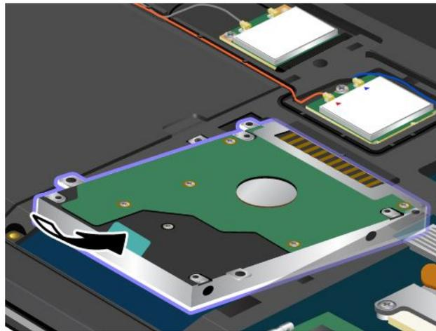
8. Slide the hard disk drive or solid-state drive firmly into the connector **1**, and then reinstall the screws **2**.
