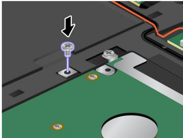
3. Reinstall the computer cover **1**. Then tighten the screws **2**.
