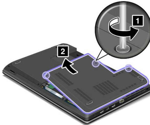
5. Remove the screws **1**, and then slide out the hard disk drive or solid-state drive **2**.
