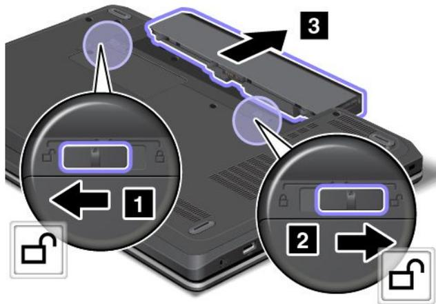
4. Insert a new battery until it clicks into place **1**, and then slide the battery latch to the locked position **2**.
