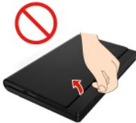
Handle the folio cover gently. The folio cover is made of genuine leather. It is not removable and is intended to protect the computer. Pulling hard will result in permanent damage to the folio cover.
