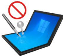
Do not scratch the screen with glass, tweezers, or any other hard or sharp objects that are not recommended to use with the ThinkPad X1 Fold Gen 1.
