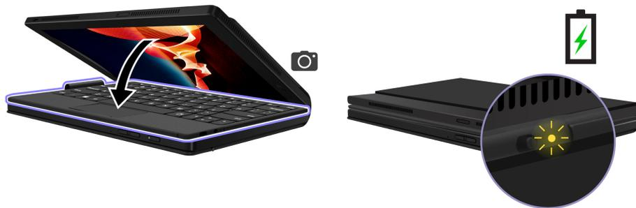
The LED indicator blinks amber three times when the keyboard is connected to computer power, then the LED indicator turns off.
