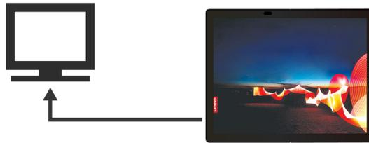
If your foldable PC cannot detect the external display, tap and hold a blank area on the desktop, and then tap **Display settings** → **Detect**.
