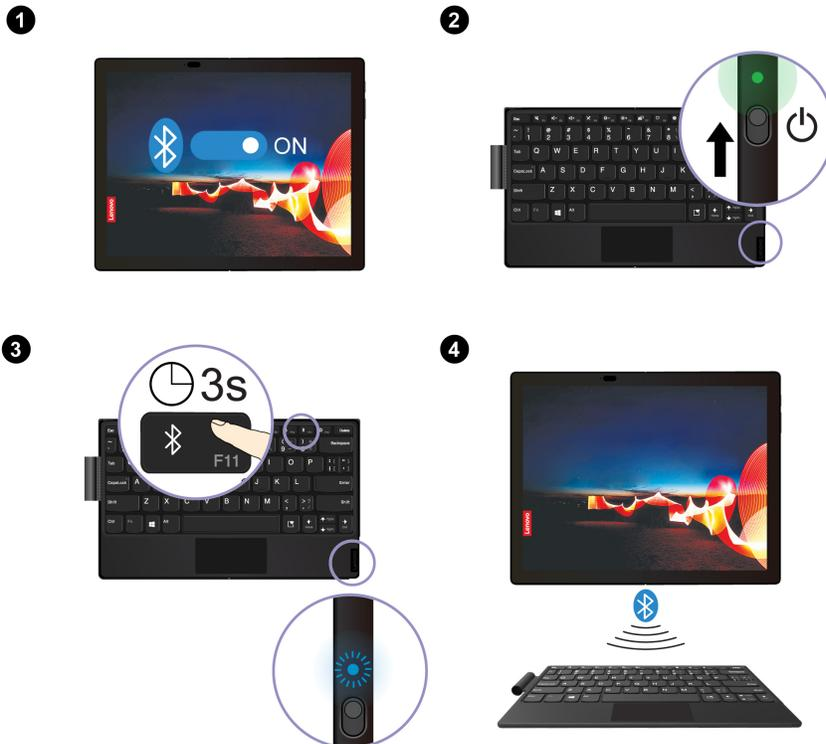
1. Enable Bluetooth function on your foldable PC. You also can enable the Swift Pair function for easy connection.
