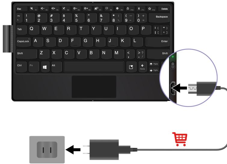
The LED indicator is in solid amber during charging and is solid green when the keyboard is fully charged.
