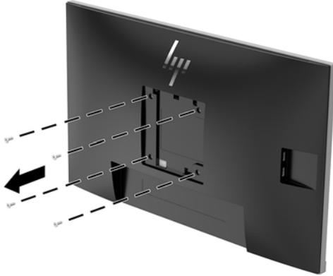
2. Install the mounting plate to the wall or swing arm of your choice using the four screws that were removed from the VESA holes on the rear of the display head.
