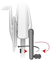
**Tip:** Make sure the different parts of the Cadence & Speed Sensor are lined up correctly on your bike. The spoke magnet should pass the main body of the chainstay sensor and the crankarm magnet should pass the tip of the sensor.
