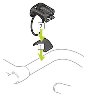
4. Wrap the O-ring around the handle bars and lift it over the back hooks.
