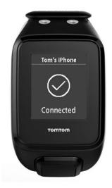
As long as you have the mobile app active or running in the background on your phone or mobile device, the watch automatically tries to connect when it has a new activity to upload or when the QuickGPSfix data is out-of-date.
