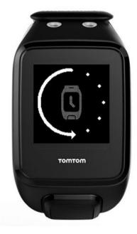
Repeat steps a-c until the compass is calibrated. When calibrated the watch gives an alert and shows a tick.
