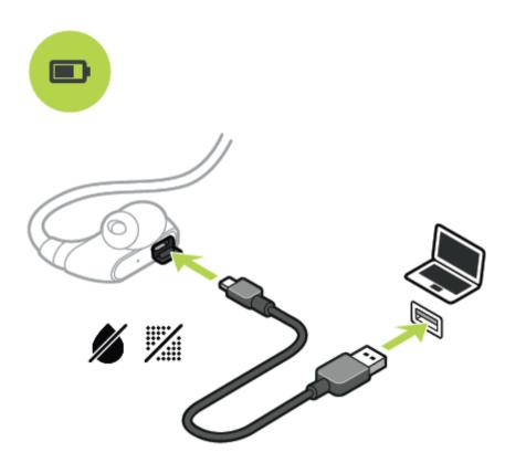
Note: When the USB socket cover is open, be careful not to get dirt, sand or water etc. in the socket.
