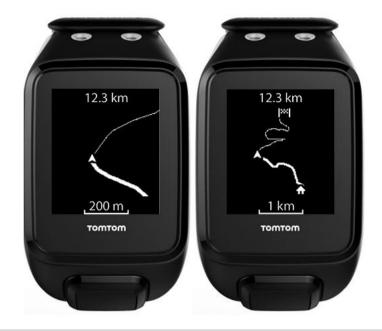
**Tip:** A scale bar is shown at the bottom of the screen and the trail orientation is always North Up.
