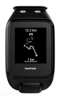
Your position is show by the arrow. The arrow tells you which direction you are facing when standing still and which direction you are headed when moving. A thicker line shows your breadcrumb trail, displaying where you have been.
