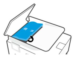
4. Pull any jammed paper out under the rollers.
