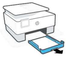
3. Check the input tray area underneath the printer. Removed the jammed paper.
