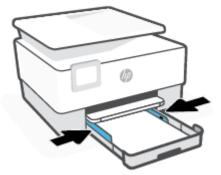
6. Reinsert the input tray into the printer.
