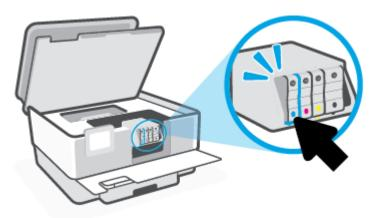
Make sure that the color-coded letter on the cartridge matches that on the slot.
