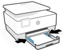
5. Reinsert the input tray into the printer.
