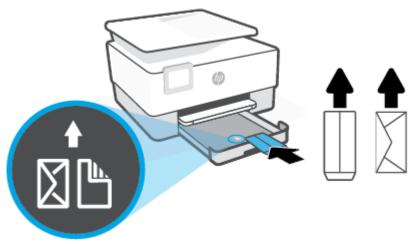
Make sure the stack of paper is aligned with the appropriate paper size lines on the front of the tray. Also, make sure the stack of paper does not exceed the stack height marking on the left edge of the tray.
