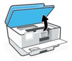
**3.** If the print carriage is not obstructed, move the print carriage to the far left of the printer and remove the jammed paper.
