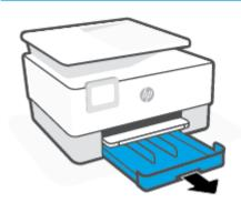
2. Slide the paper-width guides to the edges of the input tray.
