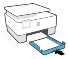
5. Insert the output tray back into the printer.
