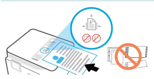
2. Slide the paper-width guides inward until they stop at the left and right edges of the paper.
