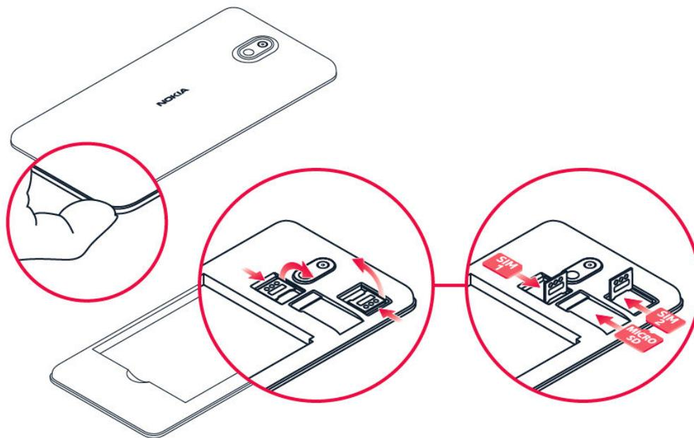
1. With the phone facing down, put your fingernail in the seam between the back cover and the display, bend the back cover open, and remove it.
