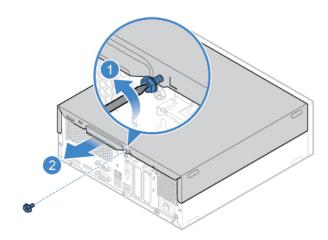
Figure 1. Removing the computer cover
