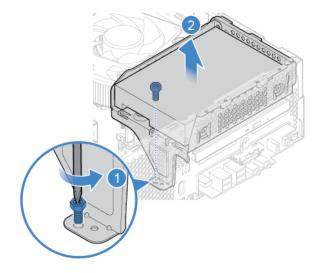
Figure 8. Removing the storage drive bracket
