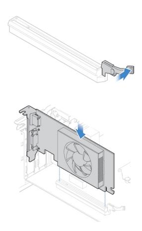
Figure 33. Installing a PCI Express card
