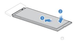
Figure 18. Installing the M.2 solid-state drive
