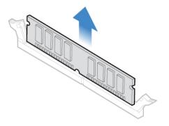
Figure 29. Removing a memory module
