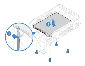
Figure 14. Installing the 2.5-inch storage drive
