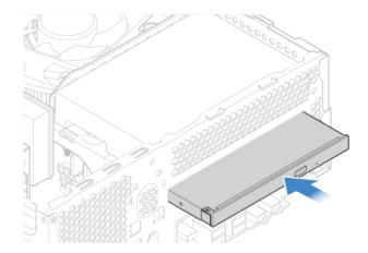
Figure 7. Installing the optical drive
