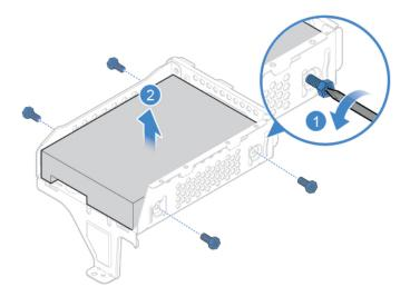
Figure 9. Removing the 3.5-inch storage drive
