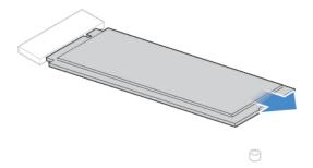
Figure 17. Removing the M.2 solid-state drive
