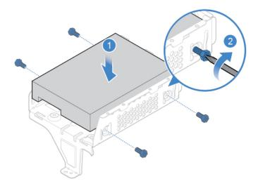
Figure 10. Installing the 3.5-inch storage drive
