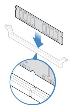
Figure 30. Installing a memory module
