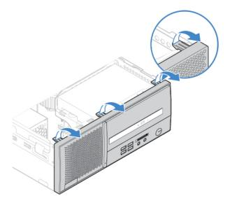
Figure 2. Removing the front bezel
