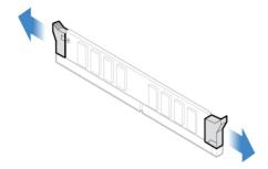
Figure 28. Disengaging the latches
