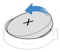
Figure 25. Removing the coin-cell battery
