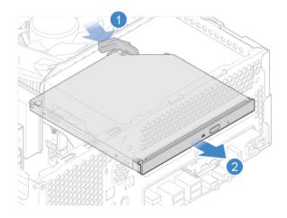
Figure 4. Removing the optical drive
