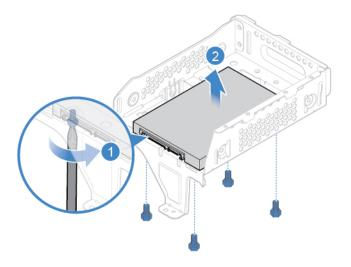
Figure 13. Removing the 2.5-inch storage drive
