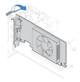
Figure 34. Securing a PCI Express card with the latch
