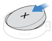
Figure 26. Installing the coin-cell battery
