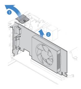
Figure 32. Removing a PCI Express card
