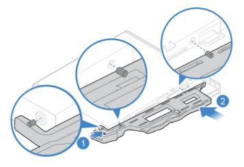
Figure 6. Installing the optical drive bracket
