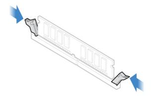
Figure 31. Securing a memory module with the latches
