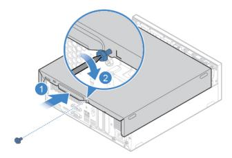
Figure 37. Reinstalling the computer cover
