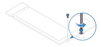
Figure 16. Removing the screw
