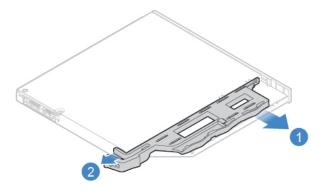
Figure 5. Removing the optical drive bracket
