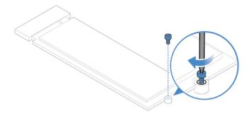
Figure 19. Installing the screw
