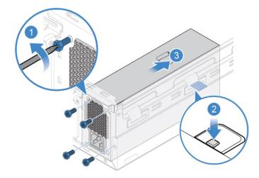
Figure 35. Removing the power supply assembly
