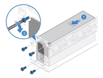
Figure 36. Installing the power supply assembly
