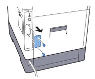
4 Insert the SD/SDHC memory card into the SD/SDHC memory card slot.
