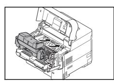
4 Insert the developer unit together with the toner container, back into the machine.
