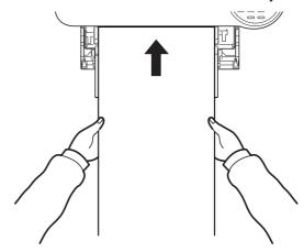
After printing starts, catch the paper when it is output so that it does not fall. When using the inner tray as the output location, do not stand up the stopper.
