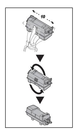
6 Shake the new toner container at least 10 times as shown in the figure in order to distribute the toner evenly inside the container. Do not press too firmly on the center of the toner container or touch the toner feed slot.
