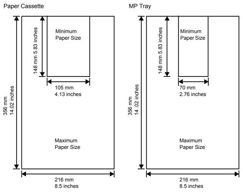
**Note** On the optional paper feeder (PF-320), the minimum size is 92 × 162 mm (3.62 × 6.38 inches) and the maximum size is 216 × 356 mm (8.5 × 14 inches).
