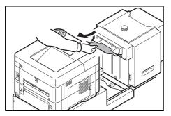
2 Remove the jammed paper from the connection opening between the Bulk Feeder and printer.
