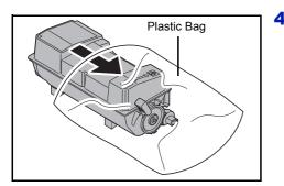
4 Put the old toner container in the plastic bag (contained in the toner kit) and discard it later according to the local code or regulations for waste disposal.
