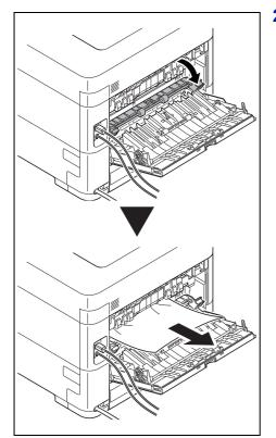
**2** Open the fuser cover and remove the jammed paper by pulling it out.
