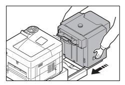
**3** Connect the Bulk Feeder to the printer.
