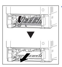
**4** Open the duplex front cover and remove any jammed paper.
