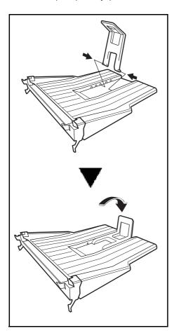
1 Install the paper stopper according to the size of paper to be used.
