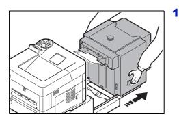
Hold the Bulk Feeder with both hands and pull out from the printer.
