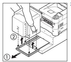
**2** Pull the Bulk Feeder out from the printer. Hold the bulk feeder with both hands and lift to remove.
