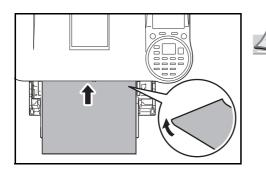
**Note** If the paper jams even after you smooth it out, load the paper in the *MP tray* with the leading edge rose up a few millimeters as shown in the illustration.
