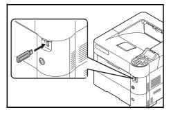
USB memory is a type of simple, highly portable flash memory that plugs into the USB memory slot. Files stored in USB memory can be printed by plugging the USB memory into the printer and then specifying the desired file names from the operation panel.
