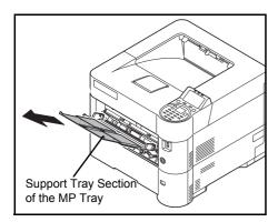
**3** Pull out the support tray section of the MP tray.
