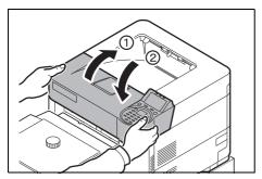
**5** After replacing the cassette in the machine and connecting the bulk feeder to the printer, open and close the top cover to clear the error. Printing will resume after the printer warms up.
