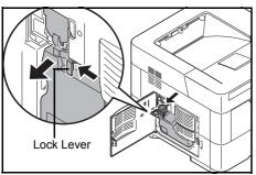
**2** While holding the waste toner box, press the lock lever and then gently remove the waste toner box.
