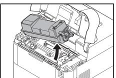
**3** Carefully remove the old toner container from the printer.
