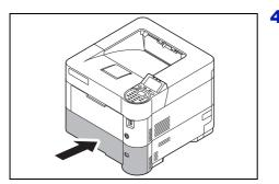
**4** Insert the cassette into the slot in the printer. The printer warms up and resumes printing.
