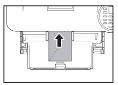
Envelopes should be fed from the MP tray with the print-side up or the optional paper feeder (PF-320) with the print-side down.
