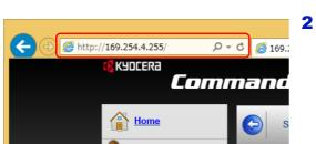
In the address or location bar, enter the machine's IP address or the host name.
