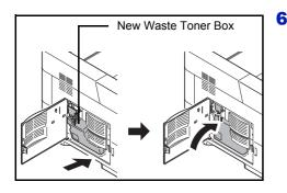
6 Insert the new waste toner box as shown in the figure. When the box is set correctly, it will snap into place.
