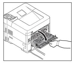
1 If paper is not completely ejected into the top tray, open the rear cover.
