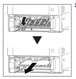
**2** Open the duplex front cover and remove any jammed paper.
