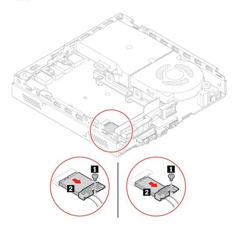
4. Remove the Wi-Fi card shield.
