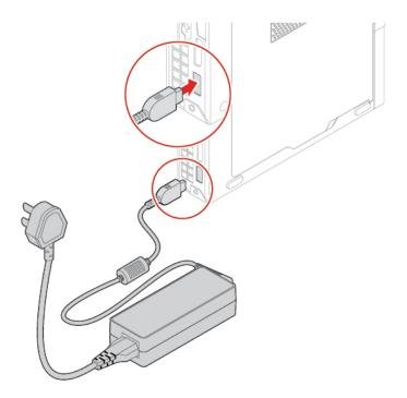
7. Reconnect the external cables and power cord to the corresponding connectors on the computer.
