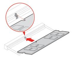
6. Secure the memory module with the latches.
