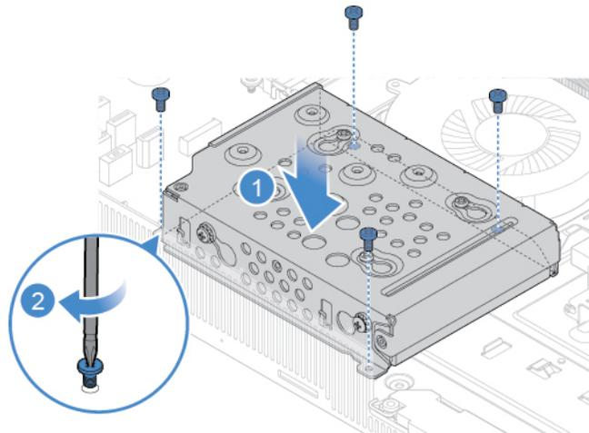
Figure 28. Installing the storage drive and the bracket
