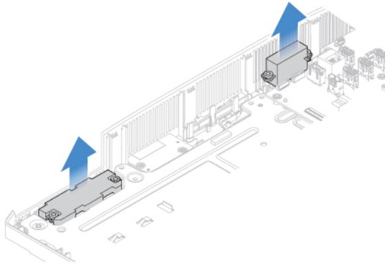
Figure 33. Removing the internal speakers
