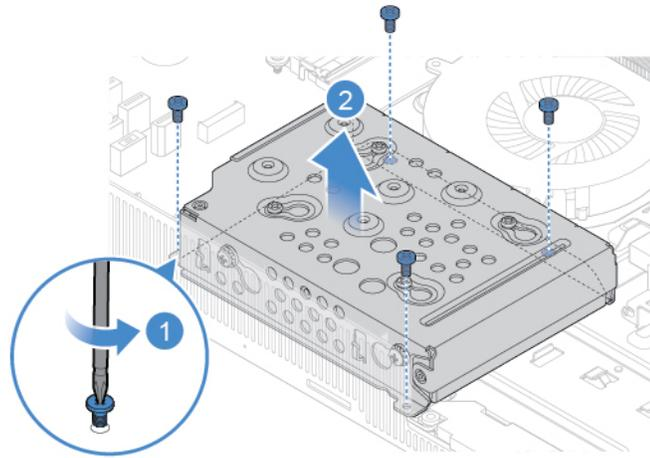
Figure 25. Removing the storage drive and the bracket
