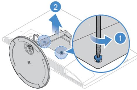
Figure 9. Removing the computer stand
