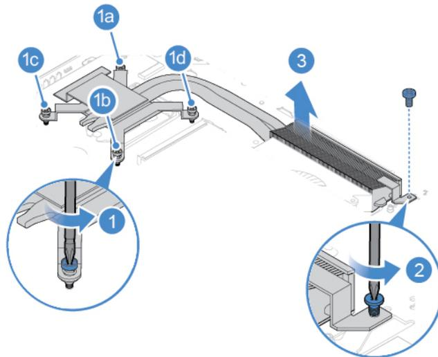
Figure 65. Removing the heat sink
