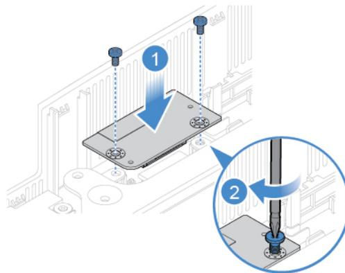
Figure 32. Installing the card reader
