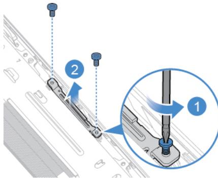
Figure 73. Removing the internal camera
