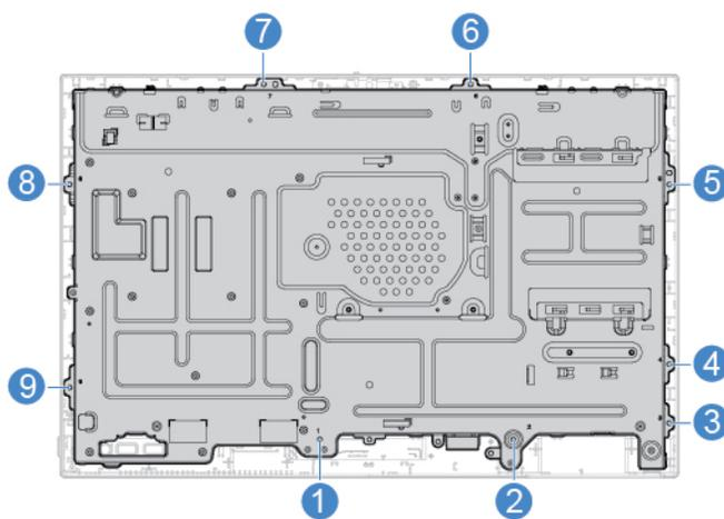
Figure 77. Removing the LCD panel and the chassis from the frame
