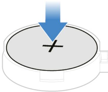
Figure 54. Securing the coin-cell battery with the latch
