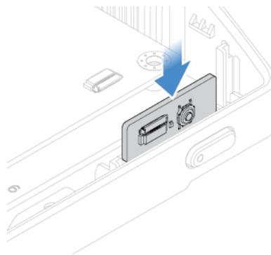
Figure 42. Installing the power button board
