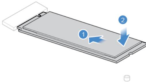
Figure 45. Installing the M.2 solid-state drive
