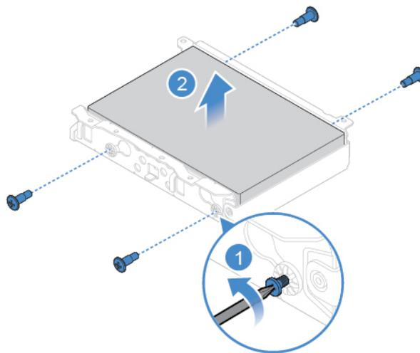
Figure 26. Removing the storage drive from the bracket
