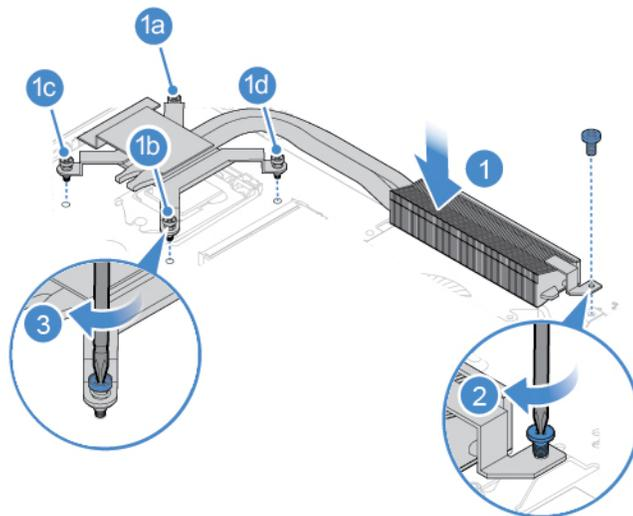
Figure 66. Installing the heat sink
