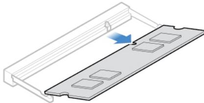
Figure 56. Removing a memory module
