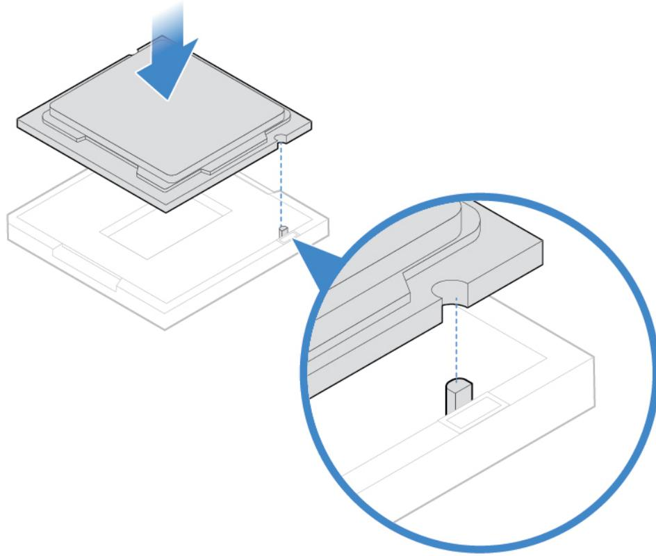
Figure 70. Installing the microprocessor
