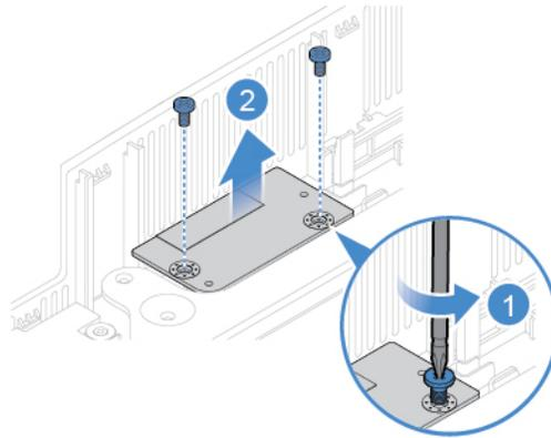
Figure 31. Removing the card reader
