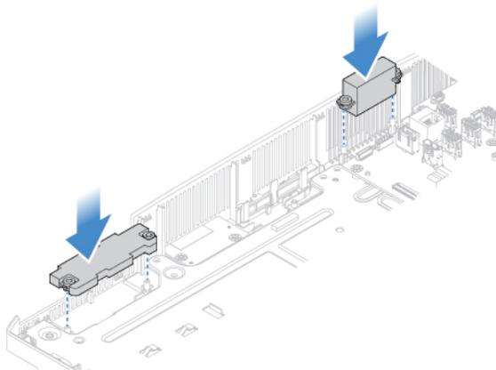
Figure 34. Installing the internal speakers
