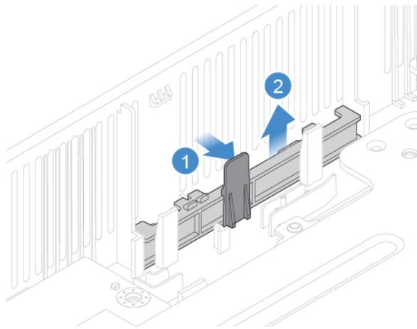
Figure 29. Removing the internal microphone board
