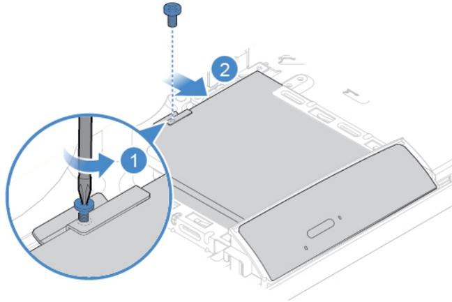
Figure 15. Removing the optical drive
