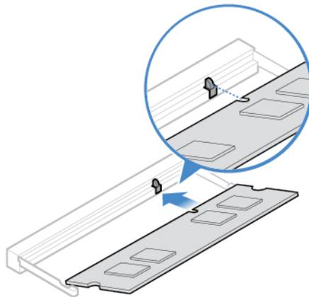
Figure 57. Installing a memory module
