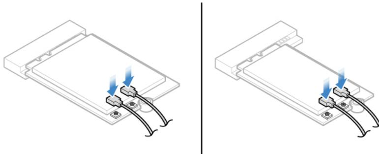
Figure 63. Connecting the Wi-Fi antenna cables
