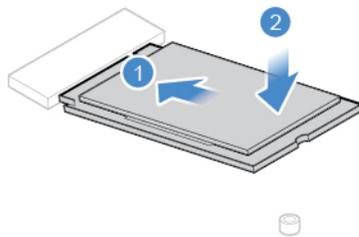
Figure 49. Installing the M.2 solid-state drive
