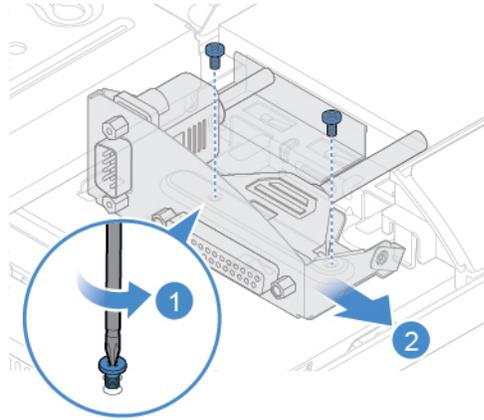
Figure 35. Removing the serial connector and parallel connector module and the bracket
