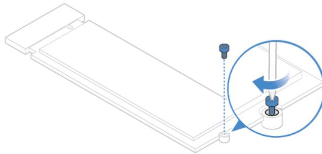
Figure 46. Installing the screw
