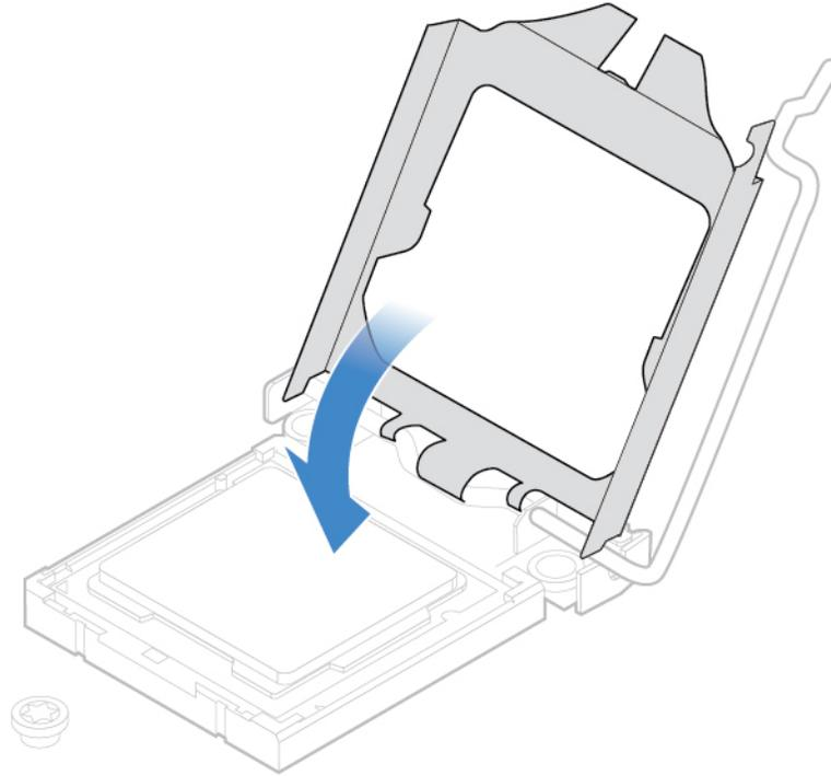
Figure 71. Closing the retainer
