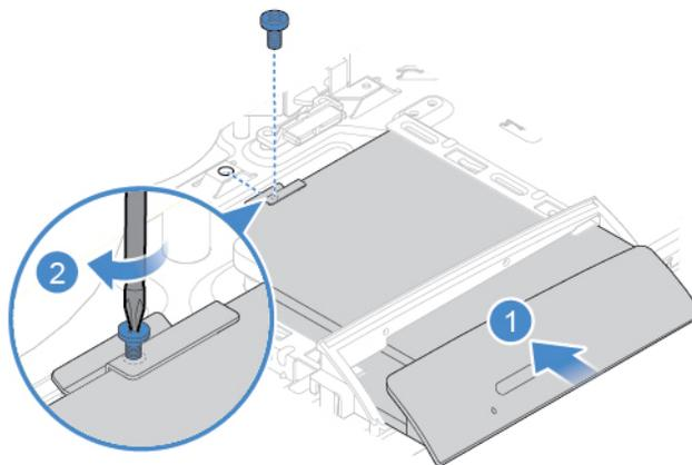
Figure 22. Installing the optical drive
