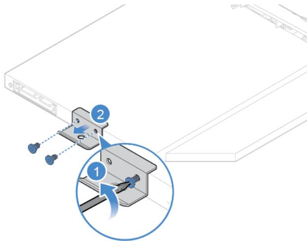
Figure 16. Removing the optical drive holder
