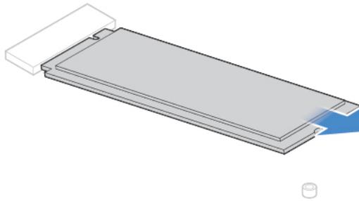
Figure 44. Removing the M.2 solid-state drive
