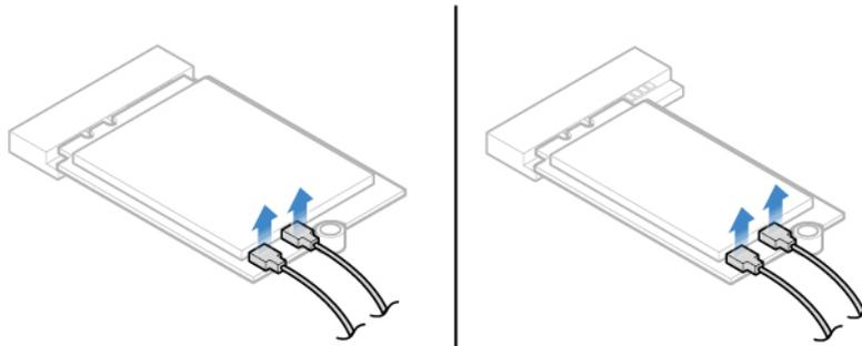
Figure 60. Disconnecting the Wi-Fi antenna cables
