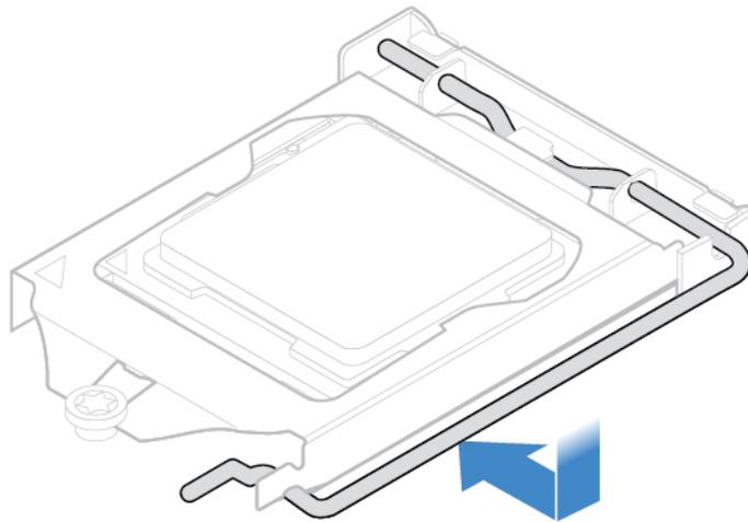
Figure 72. Securing the retainer with the handle
