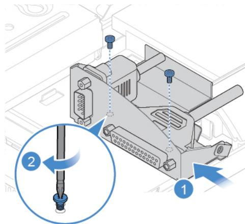
Figure 38. Installing the serial connector and parallel connector module and the bracket
