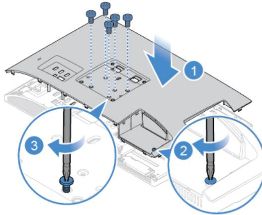
Figure 81. Installing the computer cover
