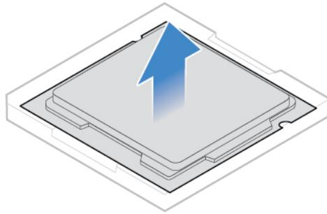
Figure 69. Removing the microprocessor
