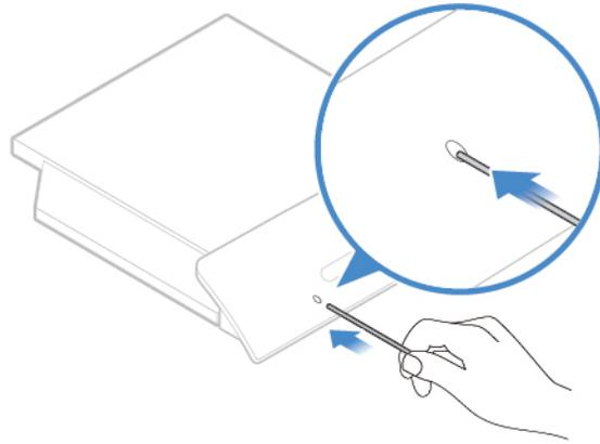
Figure 17. Inserting a straightened paper clip into the emergency-eject hole until the tray slides out
