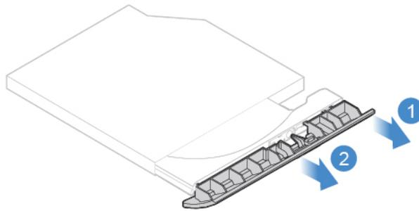
Figure 18. Removing the optical drive bezel
