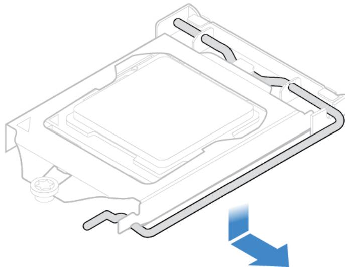
Figure 67. Releasing the handle
