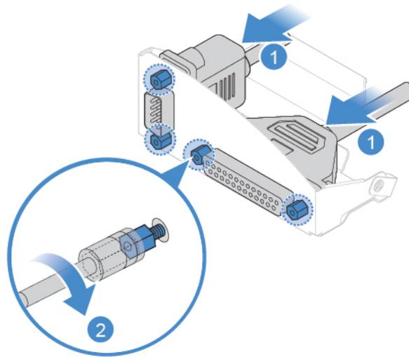
Figure 37. Installing the serial connector and parallel connector module into the bracket
