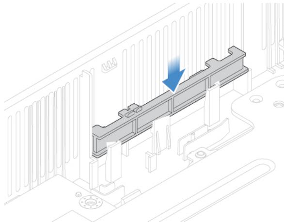
Figure 30. Installing the internal microphone board
