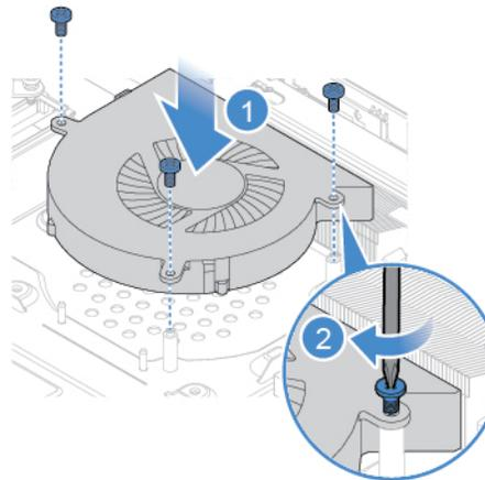
Figure 40. Installing the system fan
