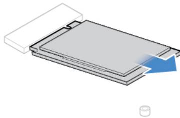
Figure 48. Removing the M.2 solid-state drive
