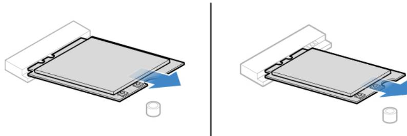
Figure 61. Removing the Wi-Fi card
