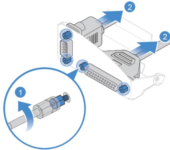
Figure 36. Removing the serial connector and parallel connector module from the bracket
