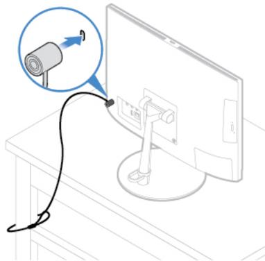
Figure 7. Attaching a Kensington-style cable lock
