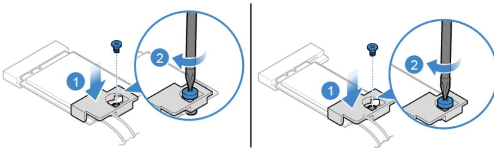
Figure 64. Installing the Wi-Fi card shield
