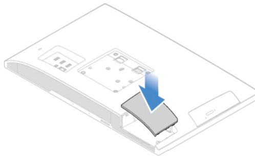
Figure 82. Installing the cover of the serial connector and parallel connector module
