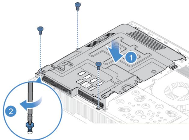
Figure 24. Installing the system board shield
