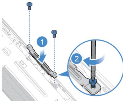
Figure 74. Installing the internal camera
