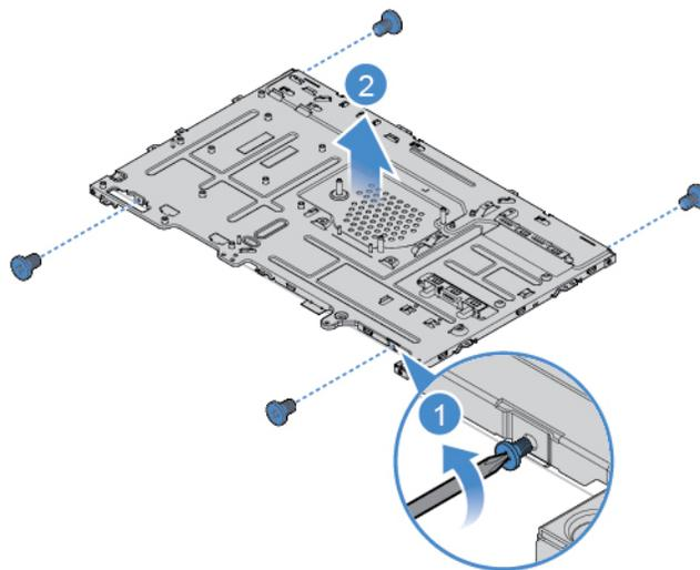
Figure 78. Removing the LCD panel from the chassis
