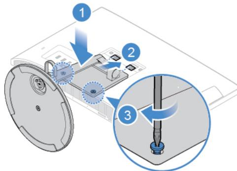
Figure 12. Installing the computer stand
