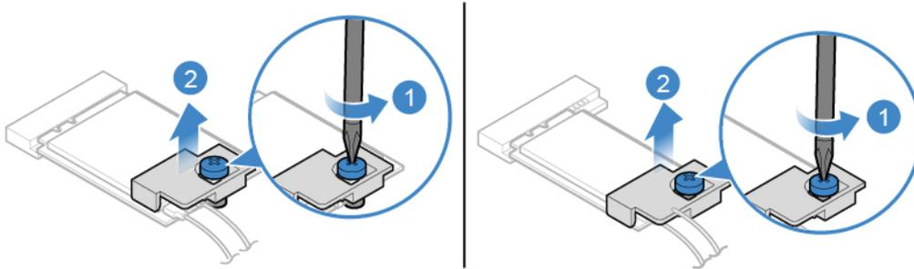
Figure 59. Removing the Wi-Fi card shield
