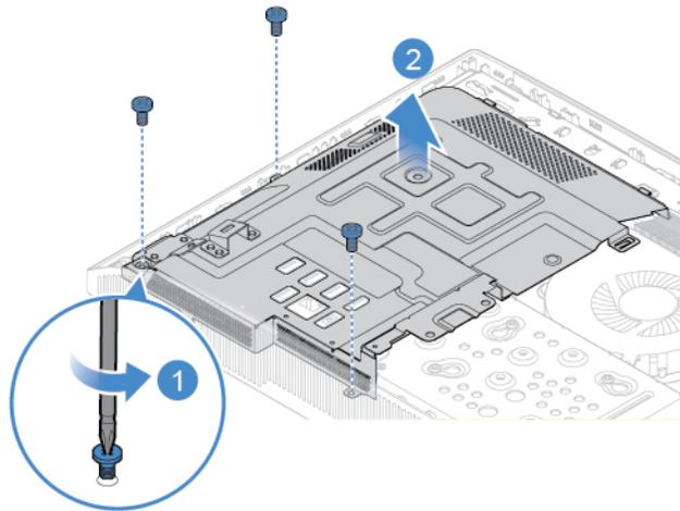
Figure 23. Removing the system board shield
