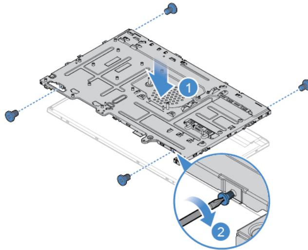
Figure 79. Installing the LCD panel into the chassis
