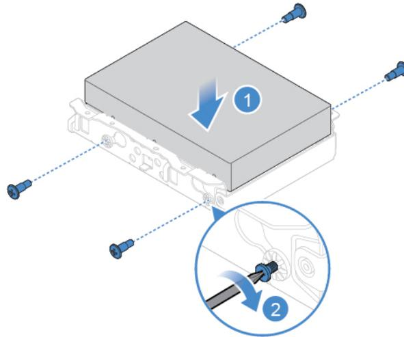
Figure 27. Installing the storage drive into the bracket
