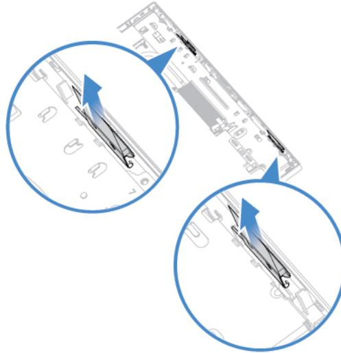
Figure 75. Removing the Wi-Fi antennas
