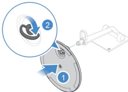
Figure 11. Installing the stand base to the stand bar
