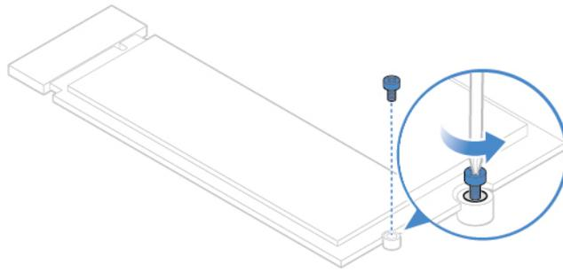
Figure 43. Removing the screw
