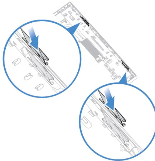
Figure 76. Installing the Wi-Fi antennas
