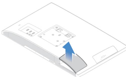
Figure 13. Removing the cover of the serial connector and parallel connector module
