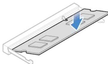
Figure 58. Securing a memory module with the latches
