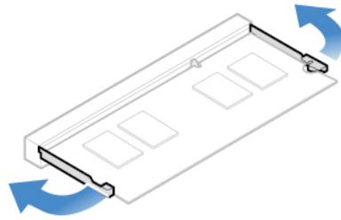
Figure 55. Disengaging the latches
