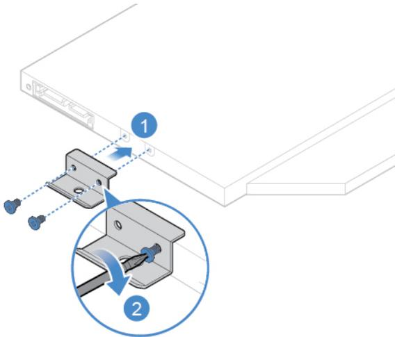
Figure 21. Installing the optical drive holder
