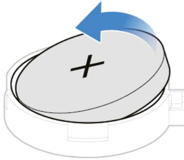
*Figure 52. Removing the coin-cell battery*
