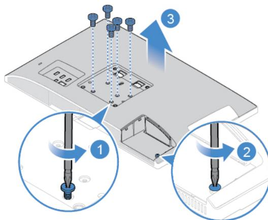
Figure 14. Removing the computer cover
