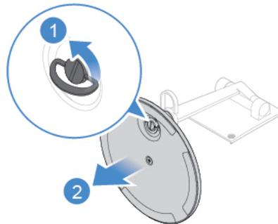
Figure 10. Removing the stand base from the stand bar
