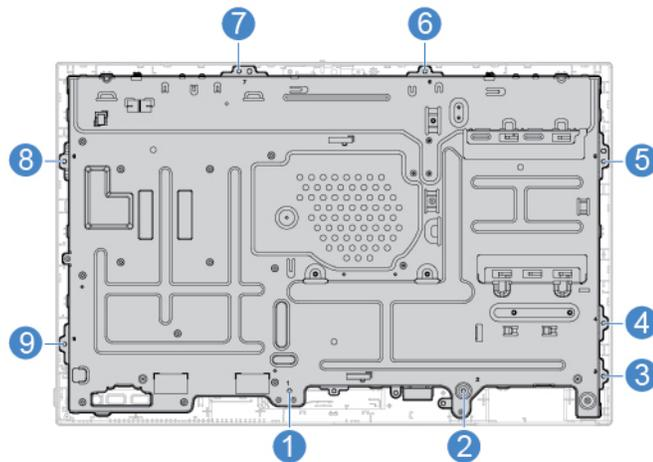
Figure 80. Installing the LCD panel and the chassis into the frame
