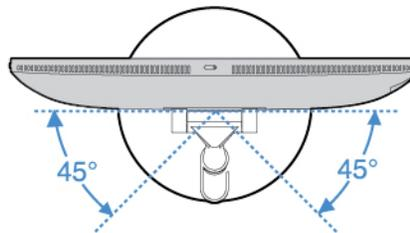
Figure 6. Turning the screen to the left and right
