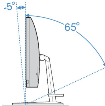
Figure 5. Tilting the screen forward and back
