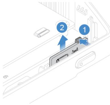
Figure 41. Removing the power button board
