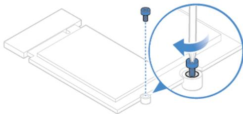
Figure 50. Installing the screw
