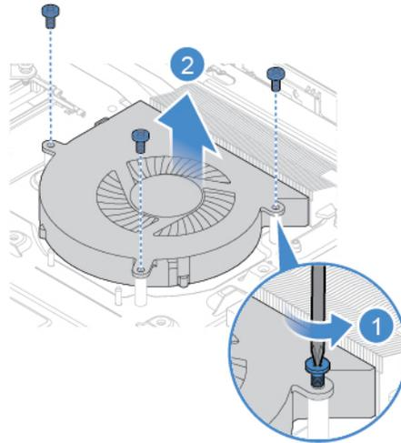
Figure 39. Removing the system fan
