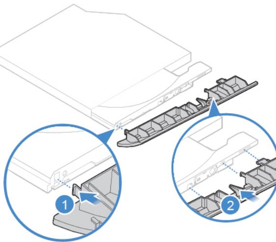
Figure 19. Installing the optical drive bezel
