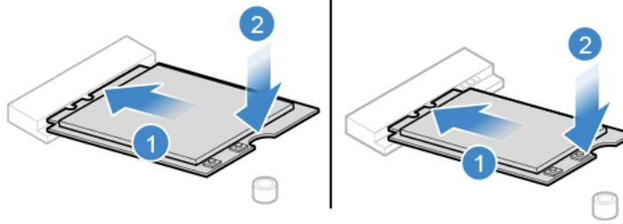
Figure 62. Installing the Wi-Fi card
