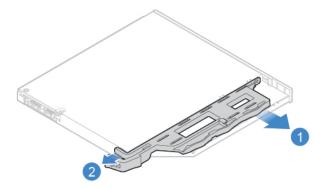
Figure 13. Removing the optical drive bracket
