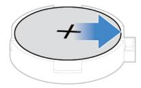
Figure 54. Disengaging the latch
