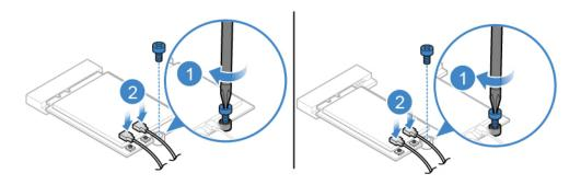
Figure 38. Connecting the Wi-Fi antenna cables
