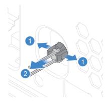
Figure 28. Removing the storage drive activity indicator
