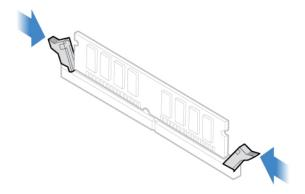
Figure 61. Securing a memory module with the latches
