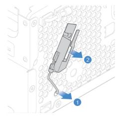
Figure 40. Removing the front Wi-Fi antenna
