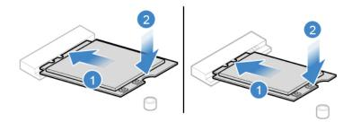
Figure 37. Installing the Wi-Fi card
