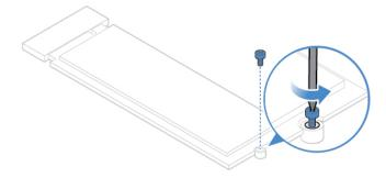
Figure 46. Removing the screw
