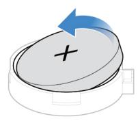
Figure 55. Removing the coin-cell battery
