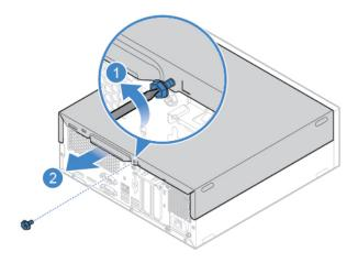
Figure 9. Removing the computer cover
