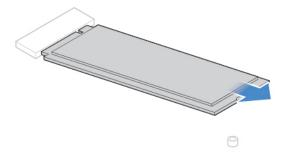
Figure 47. Removing the M.2 solid-state drive
