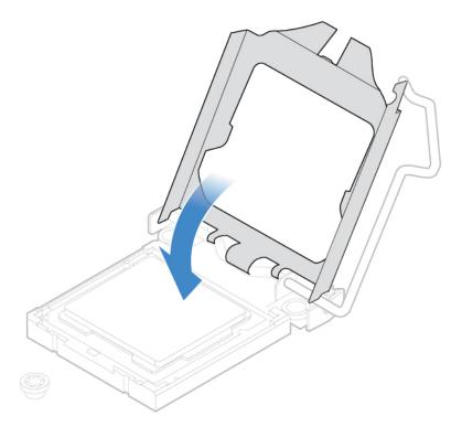
Figure 68. Closing the retainer
