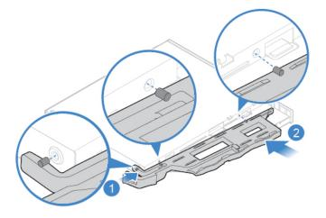
Figure 14. Installing the optical drive bracket
