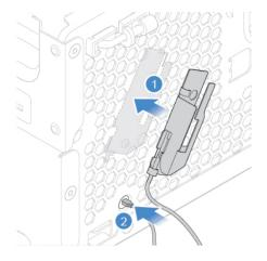
Figure 41. Installing the front Wi-Fi antenna
