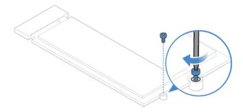
Figure 49. Installing the screw
