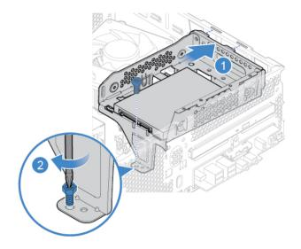
Figure 23. Installing the storage drive bracket
