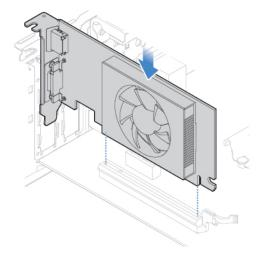
Figure 71. Installing a PCI Express card
