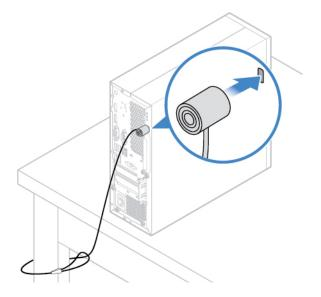
Figure 6. Attaching a Kensington-style cable lock
