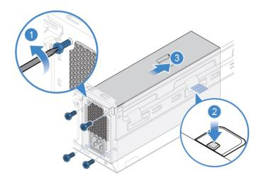
Figure 73. Removing the power supply assembly
