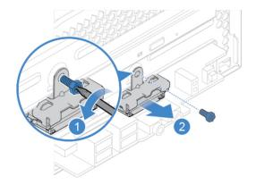
Figure 24. Removing the card reader bracket
