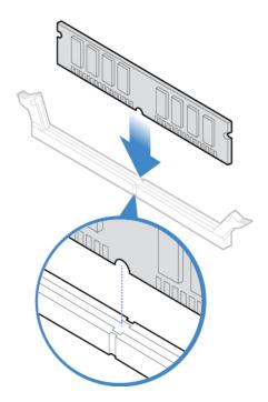
Figure 60. Installing a memory module
