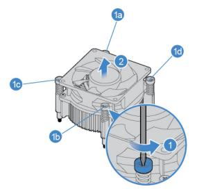
Figure 62. Removing the heat sink and fan assembly
