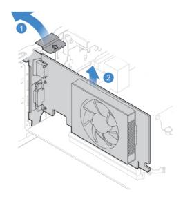
Figure 70. Removing a PCI Express card
