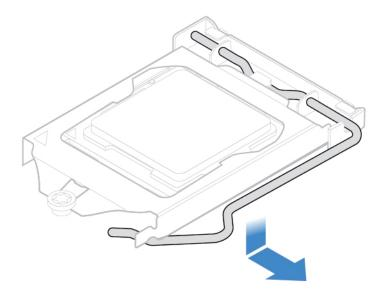
Figure 64. Releasing the handle
