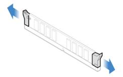
Figure 58. Disengaging the latches
