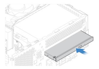
Figure 15. Installing the optical drive
