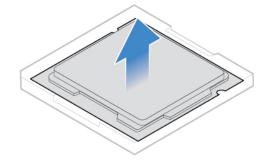
Figure 66. Removing the microprocessor
