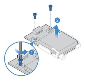
Figure 25. Removing the card reader
