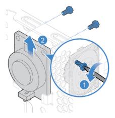
Figure 30. Removing the internal speaker
