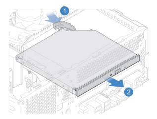
Figure 12. Removing the optical drive
