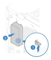
Figure 42. Removing the rear Wi-Fi antenna cover
