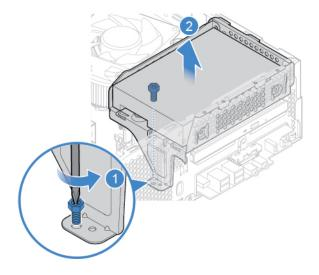
Figure 16. Removing the storage drive bracket
