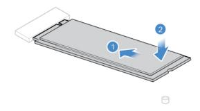
Figure 48. Installing the M.2 solid-state drive
