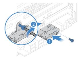
Figure 27. Installing the card reader bracket
