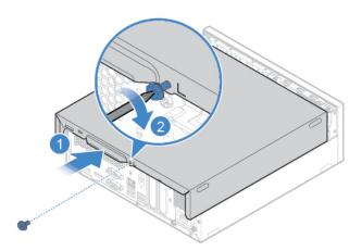
Figure 75. Reinstalling the computer cover
