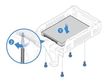
Figure 22. Installing the 2.5-inch storage drive
