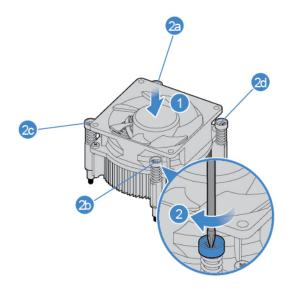
Figure 63. Installing the heat sink and fan assembly
