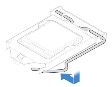
Figure 69. Securing the retainer with the handle
