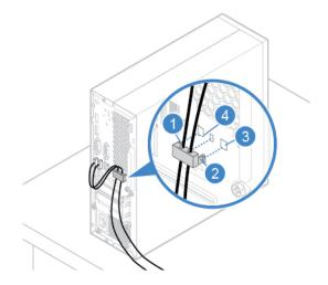
Figure 7. Attaching a smart cable clip
