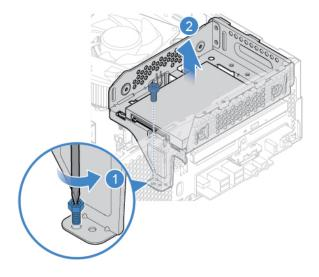
Figure 20. Removing the storage drive bracket
