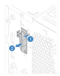
Figure 43. Removing the rear Wi-Fi antenna
