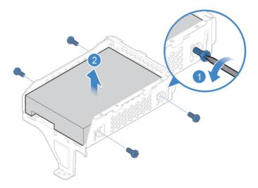
Figure 17. Removing the 3.5-inch storage drive
