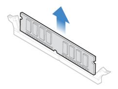
Figure 59. Removing a memory module
