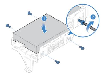
Figure 18. Installing the 3.5-inch storage drive
