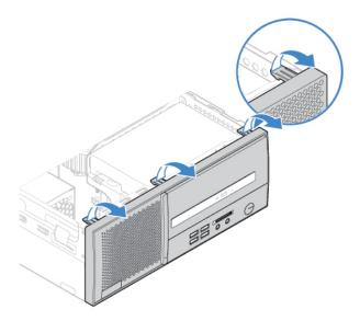
Figure 10. Removing the front bezel
