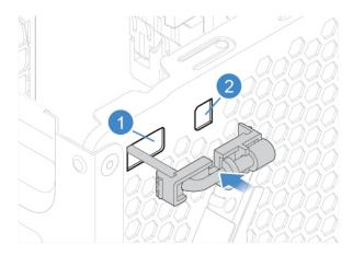
Figure 33. Installing the thermal sensor
