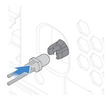
Figure 29. Installing the storage drive activity indicator
