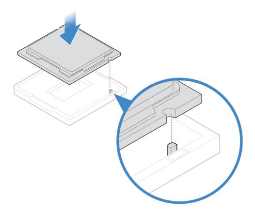
Figure 67. Installing the microprocessor
