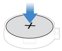
Figure 57. Securing the coin-cell battery with the latch
