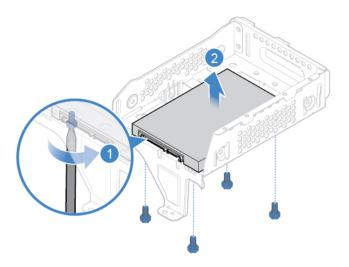
Figure 21. Removing the 2.5-inch storage drive
