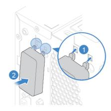
Figure 45. Installing the rear Wi-Fi antenna cover
