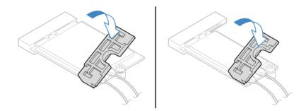
Figure 39. Installing the Wi-Fi card shield
