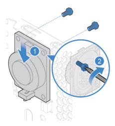
Figure 31. Installing the internal speaker
