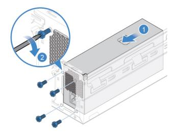
Figure 74. Installing the power supply assembly
