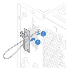
Figure 44. Installing the rear Wi-Fi antenna
