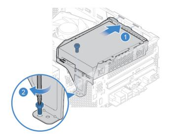
Figure 19. Installing the storage drive bracket
