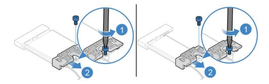
Figure 34. Removing the Wi-Fi card shield
