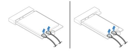
Figure 35. Disconnecting the Wi-Fi antenna cables
