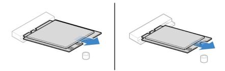
Figure 36. Removing the Wi-Fi card
