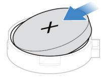
Figure 56. Installing the coin-cell battery
