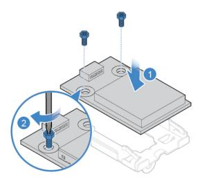
Figure 26. Installing the card reader
