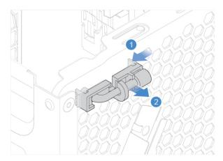
Figure 32. Removing the thermal sensor
