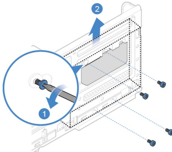
Figure 19. Removing the 3.5-inch secondary storage drive
