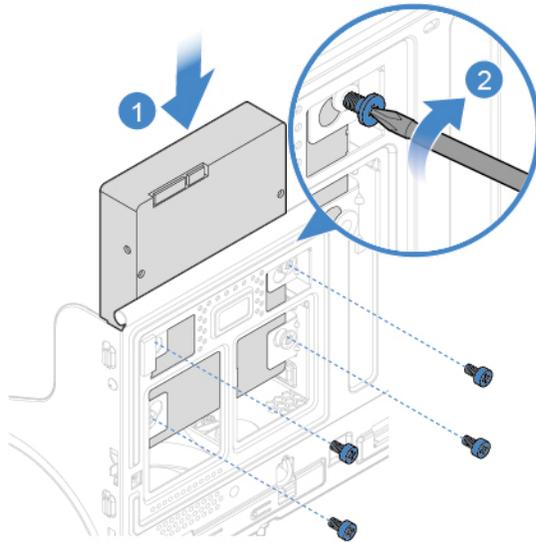
Figure 18. Installing the 3.5-inch primary storage drive
