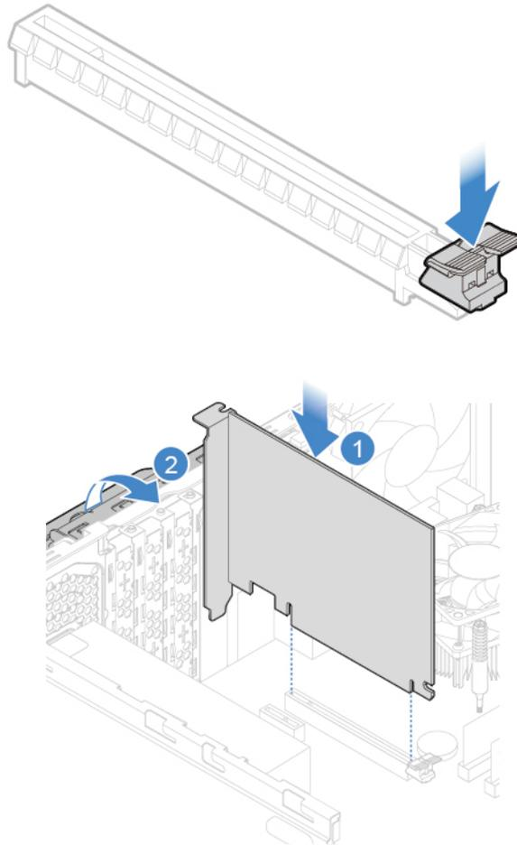
Figure 34. Installing a PCI Express card
