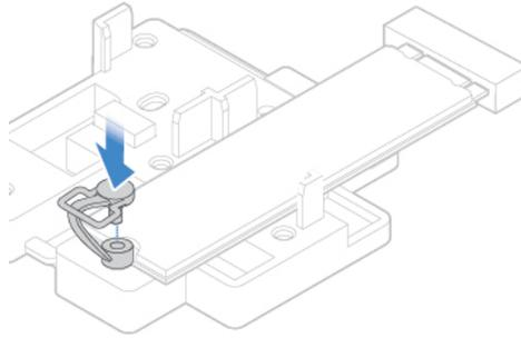
Figure 50. Inserting the stopper
