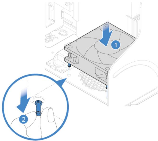
Figure 64. Installing the front fan
