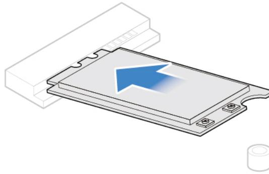
Figure 44. Installing the Wi-Fi card
