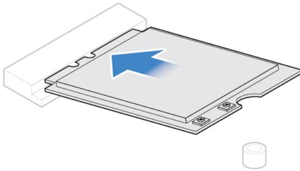
Figure 38. Installing the Wi-Fi card
