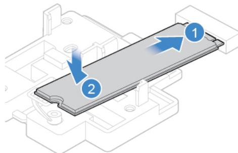
Figure 49. Installing the M.2 solid-state drive
