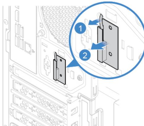
Figure 68. Removing the rear Wi-Fi antenna
