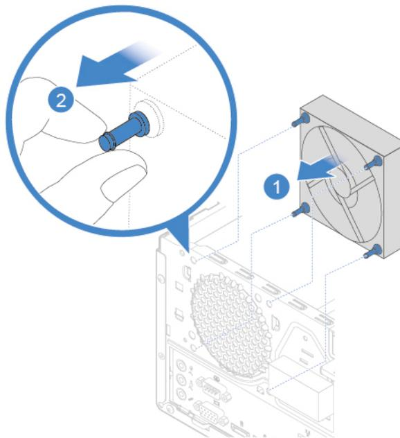
Figure 87. Installing the rear fan
