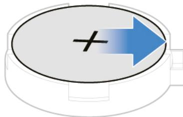
*Figure 29. Disengaging the latch*
