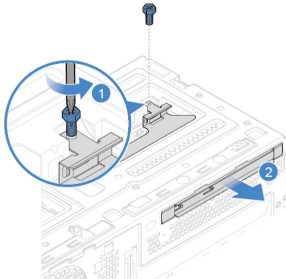
Figure 13. Removing the optical drive bracket
