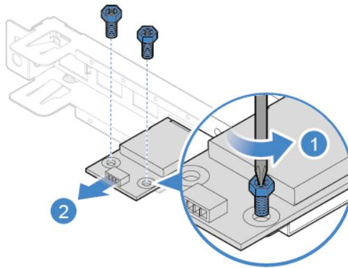
Figure 77. Removing the card reader
