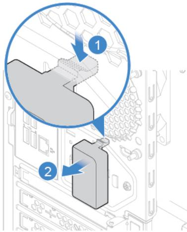
Figure 67. Removing the rear Wi-Fi antenna cover
