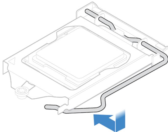
Figure 85. Securing the retainer with the handle
