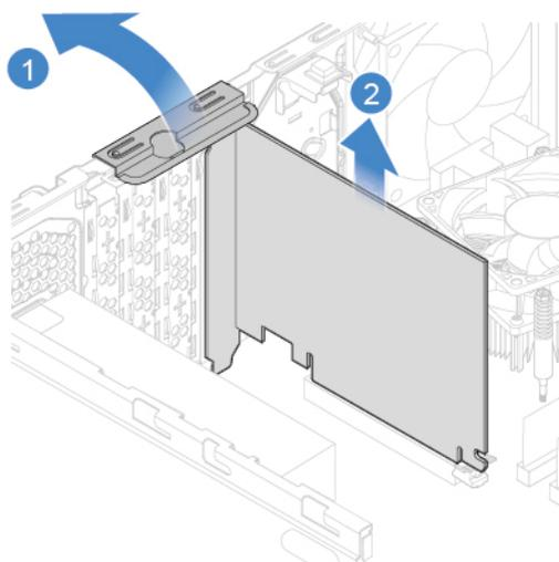
Figure 33. Removing a PCI Express card
