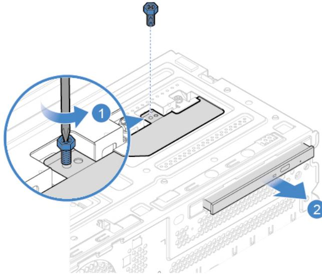
Figure 11. Removing the optical drive
