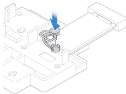
Figure 54. Inserting the stopper
