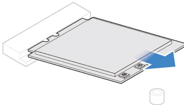
Figure 37. Removing the Wi-Fi card
