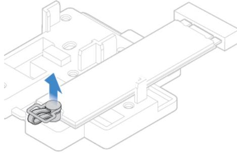
Figure 47. Pulling out the stopper
