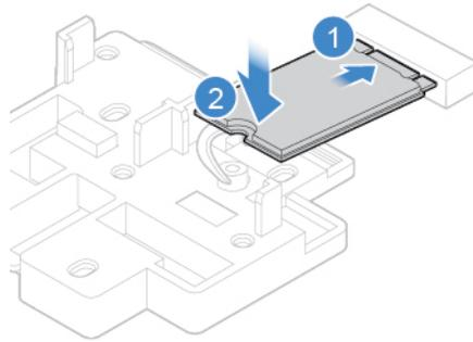
Figure 53. Installing the M.2 solid-state drive
