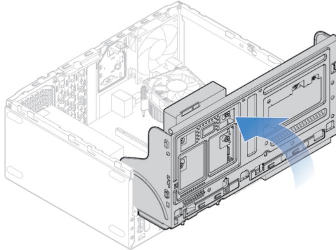
Figure 75. Pivoting the drive bay assembly downward
