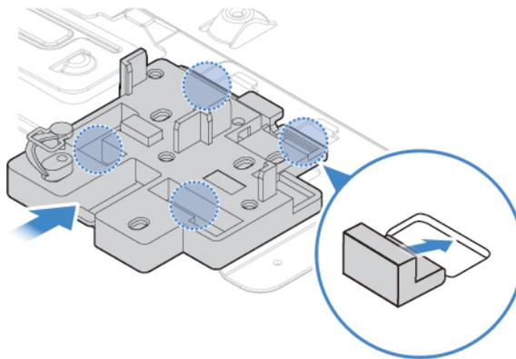
Figure 56. Installing the M.2 solid-state drive bracket
