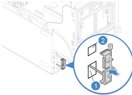
Figure 62. Installing the thermal sensor
