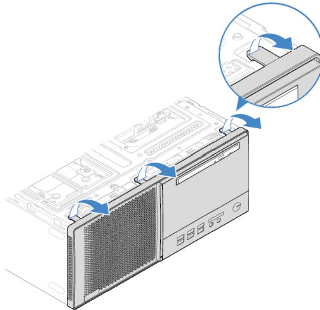
Figure 9. Removing the front bezel
