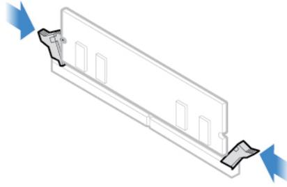
Figure 26. Securing a memory module with the latches
