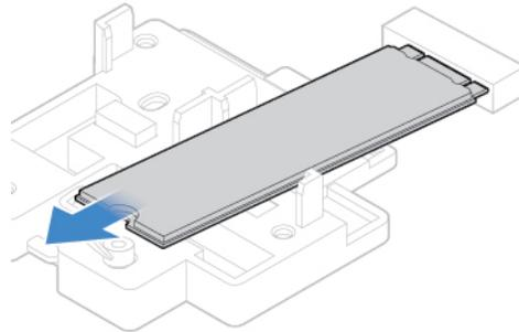
Figure 48. Removing the M.2 solid-state drive
