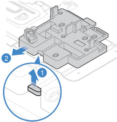
Figure 55. Removing the M.2 solid-state drive bracket
