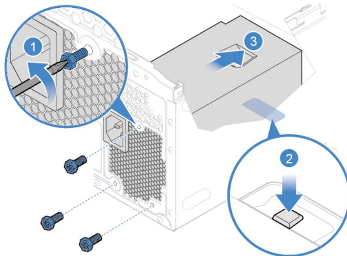
*Figure 57. Removing the power supply assembly*
