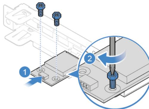
Figure 78. Installing the card reader
