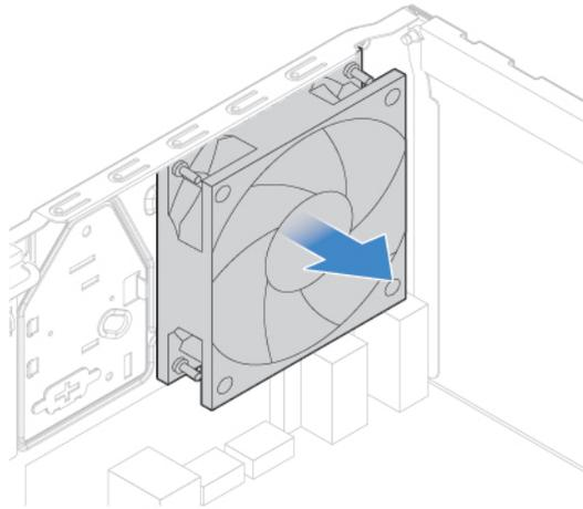
Figure 86. Removing the rear fan
