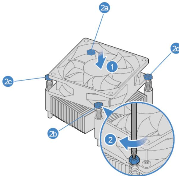
Figure 28. Installing the heat sink and fan assembly
