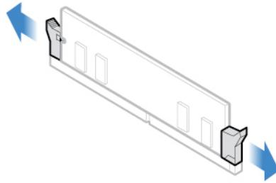
Figure 23. Disengaging the latches
