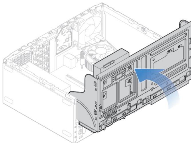
Figure 16. Pivoting the drive bay assembly downward
