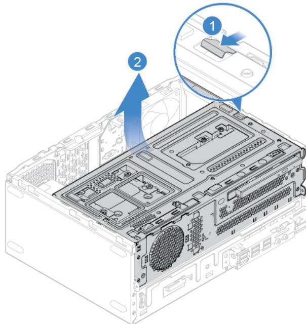
Figure 72. Pivoting the drive bay assembly upward
