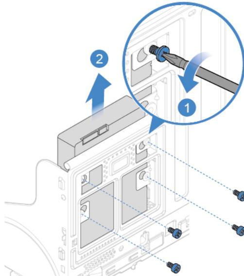
Figure 17. Removing the 3.5-inch primary storage drive
