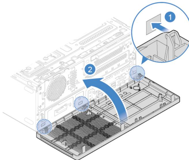
Figure 10. Installing the front bezel
