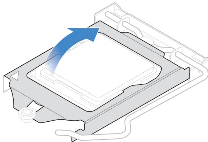
Figure 81. Opening the retainer
