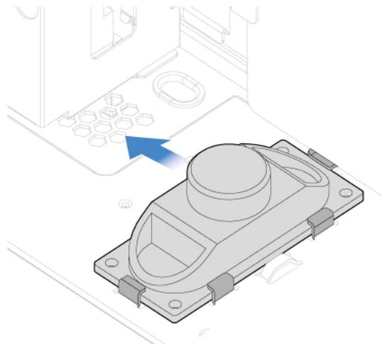
Figure 59. Removing the internal speaker
