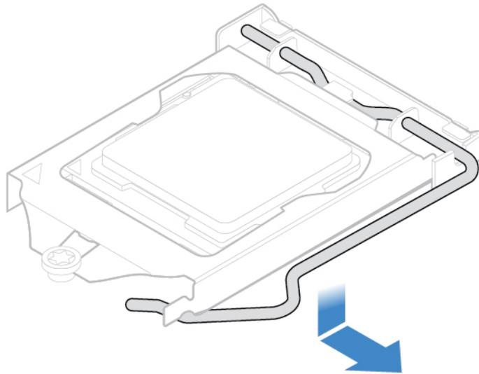
Figure 80. Releasing the handle
