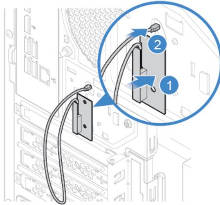
Figure 69. Installing the rear Wi-Fi antenna
