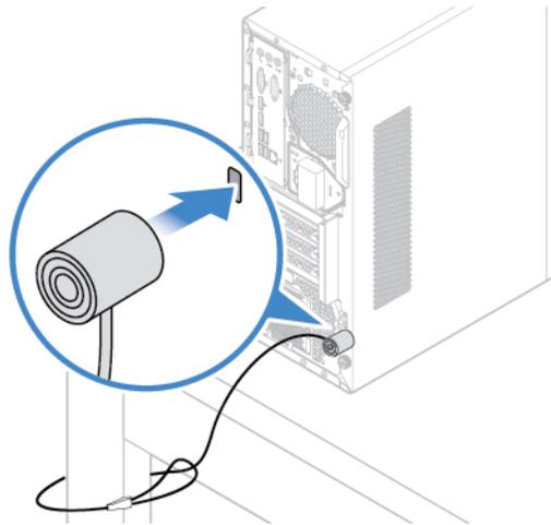
Figure 6. Attaching a Kensington-style cable lock
