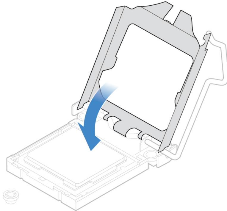
Figure 84. Closing the retainer
