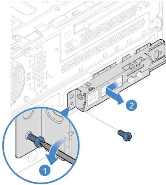
Figure 76. Removing the front I/O bracket
