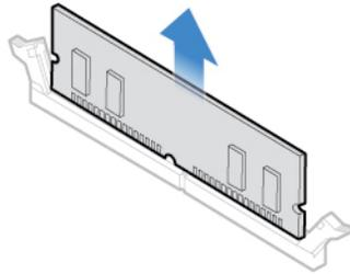
Figure 24. Removing a memory module
