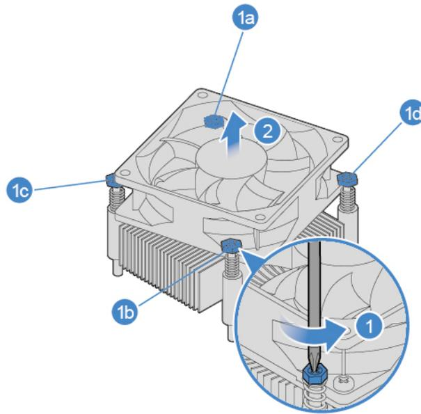
Figure 27. Removing the heat sink and fan assembly
