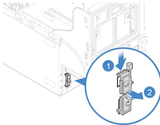
Figure 61. Removing the thermal sensor
