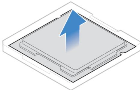
Figure 82. Removing the microprocessor
