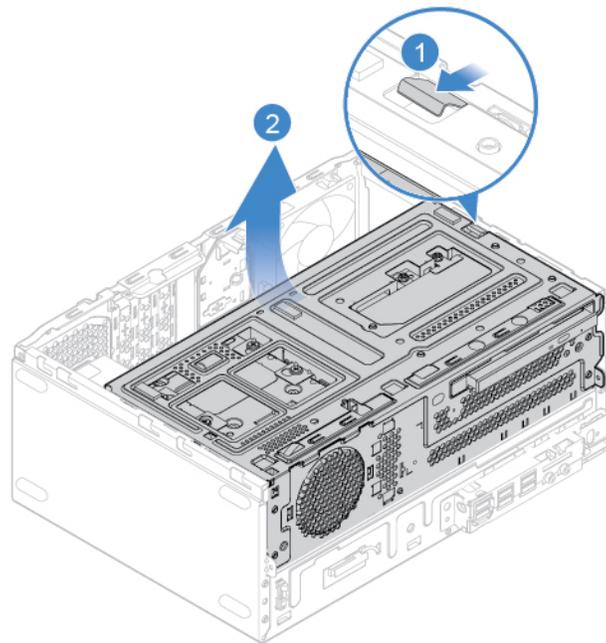
Figure 15. Pivoting the drive bay assembly upward
