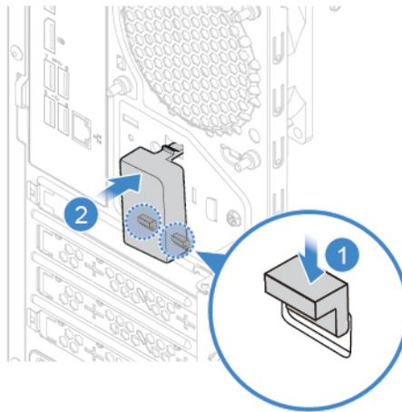
Figure 70. Installing the rear Wi-Fi antenna cover
