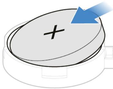
*Figure 31. Installing the coin-cell battery*
