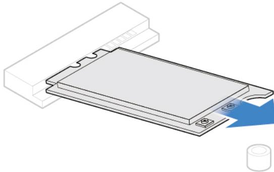
Figure 43. Removing the Wi-Fi card
