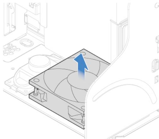
Figure 63. Removing the front fan
