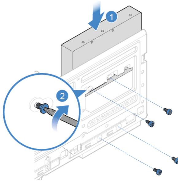
Figure 20. Installing the 3.5-inch secondary storage drive
