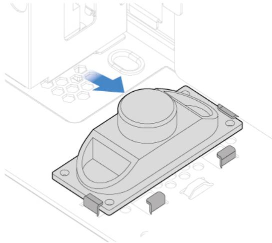
Figure 60. Installing the internal speaker
