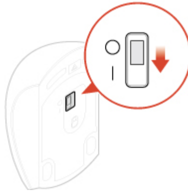
Figure 18. Pushing the power switch to the ON position
