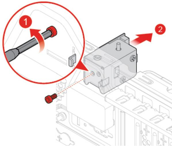
Figure 125. Removing the E-lock
