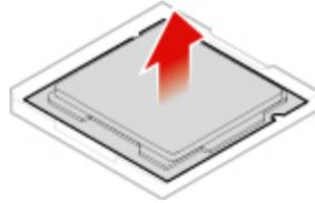
Figure 114. Removing the microprocessor
