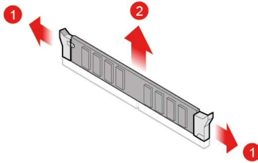
Figure 42. Removing the memory module
