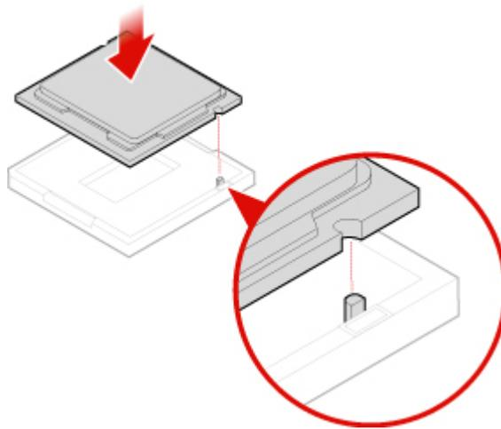
Figure 115. Installing the microprocessor
