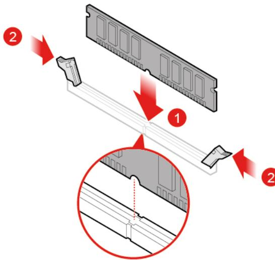
Figure 43. Installing the memory module
