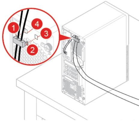
Figure 8. Attaching a smart cable clip
