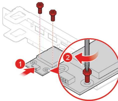
Figure 106. Installing the card reader board
