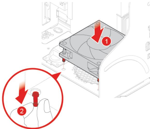
Figure 89. Installing the front fan
