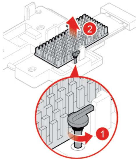
Figure 64. Removing the M.2 solid-state drive heat sink
