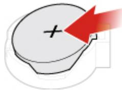
Figure 122. Placing the coin-cell battery
