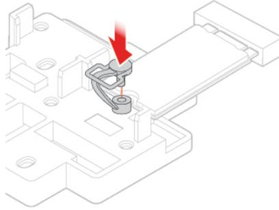
Figure 68. Locking the M.2 solid-state drive clip
