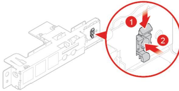
Figure 103. Removing the power button
