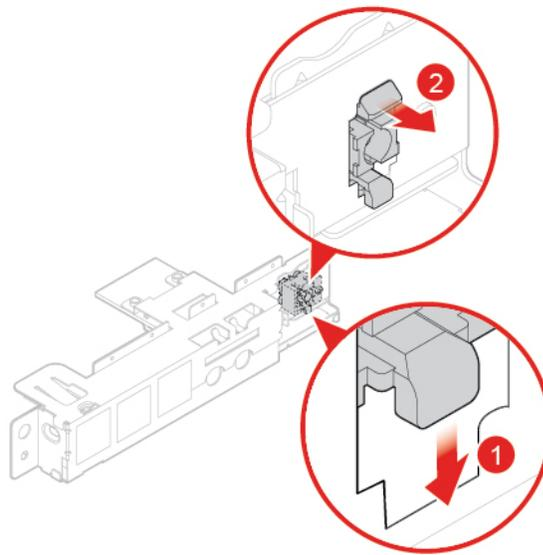
Figure 104. Installing the power button
