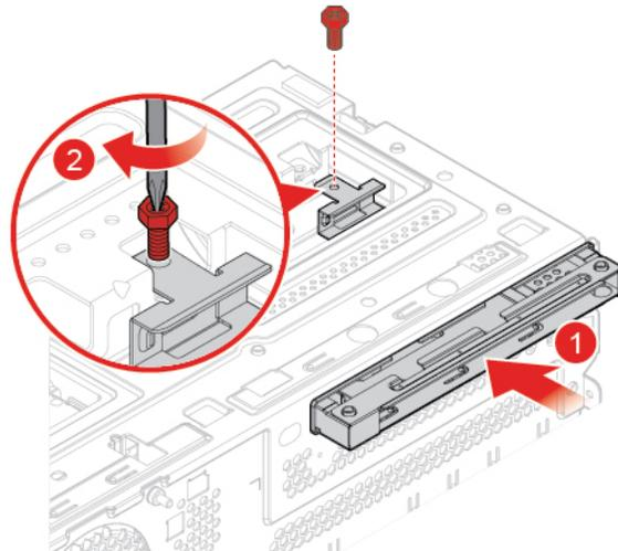
Figure 29. Installing the optical drive bracket
