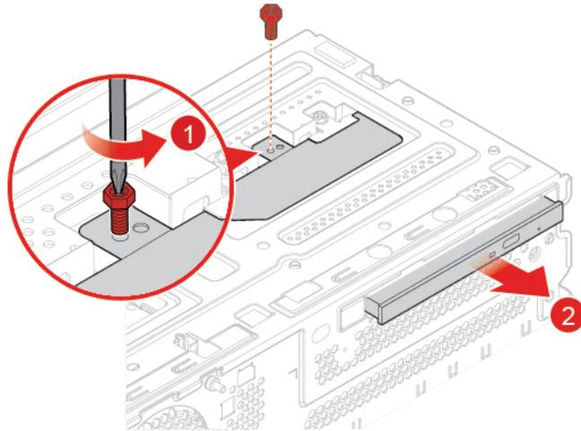
Figure 26. Removing the optical drive
