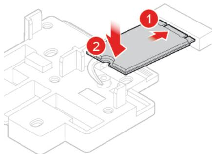
Figure 67. Installing the M.2 solid-state drive
