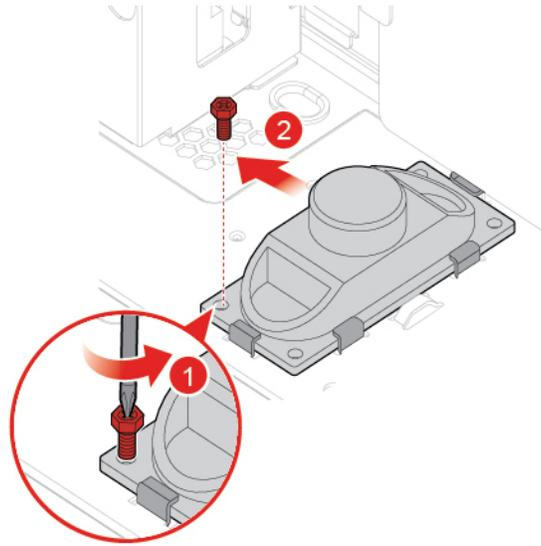
Figure 84. Removing the internal speaker
