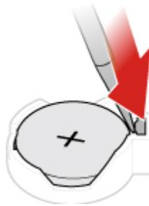
Figure 120. Pressing the metallic tab using a driver
