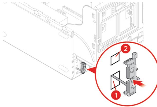
Figure 97. Installing the thermal sensor
