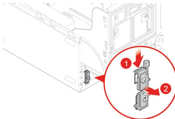
Figure 96. Removing the thermal sensor
