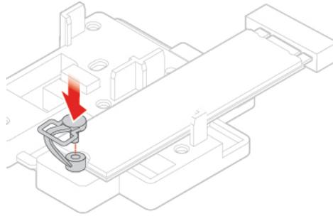
Figure 60. Locking the M.2 solid-state drive clip
