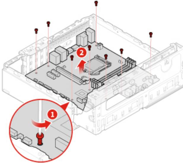
Figure 133. Removing the system board
