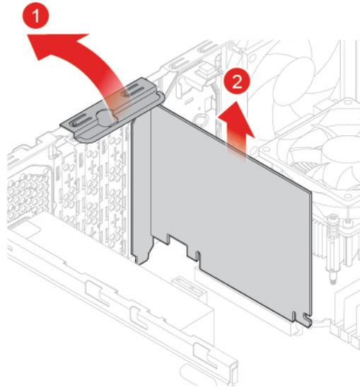
Figure 46. Removing the PCI Express card
