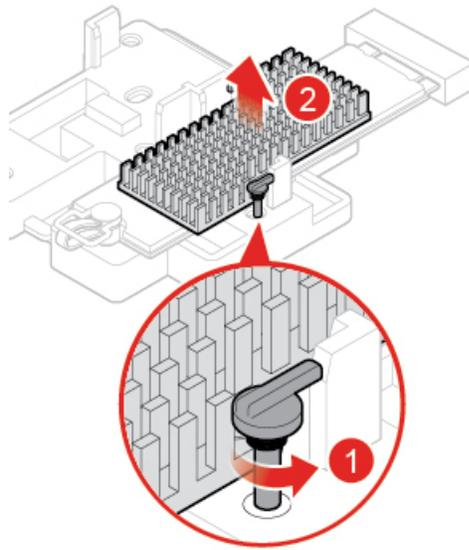
Figure 56. Removing the M.2 solid-state drive heat sink
