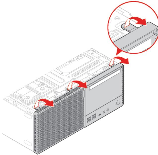
Figure 24. Removing the front bezel
