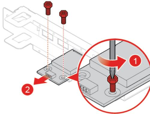
Figure 105. Removing the card reader board
