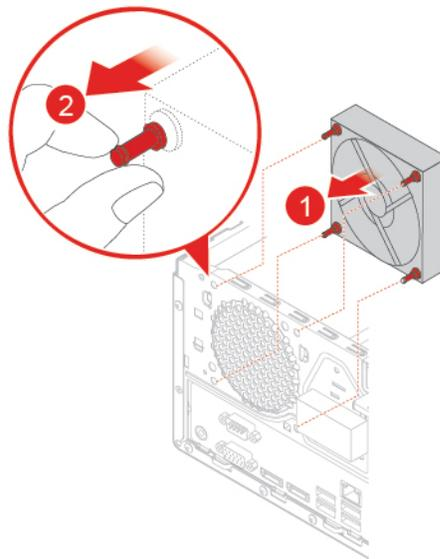
Figure 132. Installing the rear fan
