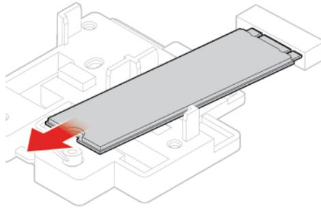
Figure 58. Removing the M.2 solid-state drive
