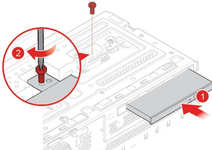
Figure 27. Installing the optical drive
