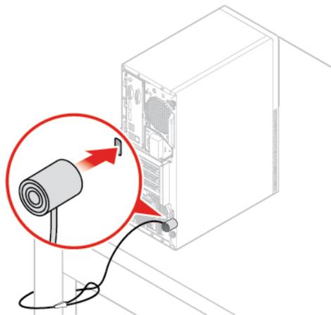
Figure 7. Attaching a Kensington-style cable lock
