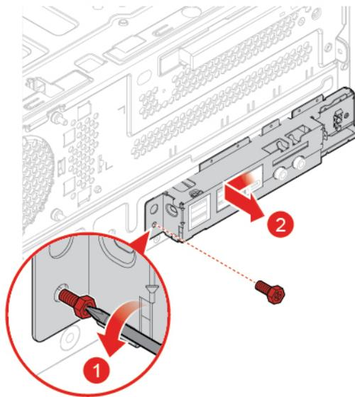
Figure 100. Removing the front I/O bracket
