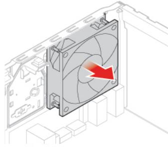
Figure 131. Removing the rear fan
