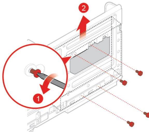
Figure 35. Removing the 3.5-inch secondary storage drive
