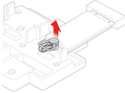
Figure 65. Unlocking the M.2 solid-state drive clip
