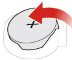
Figure 121. Removing the coin-cell battery
