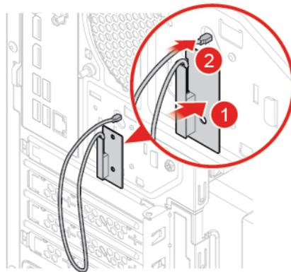
Figure 81. Installing the rear Wi-Fi antenna
