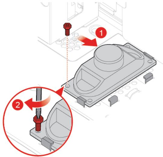
Figure 85. Installing the internal speaker
