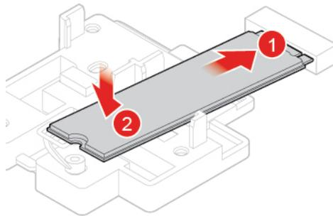
Figure 59. Installing the M.2 solid-state drive
