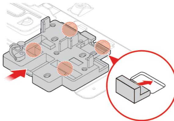
Figure 72. Installing the M.2 solid-state drive bracket
