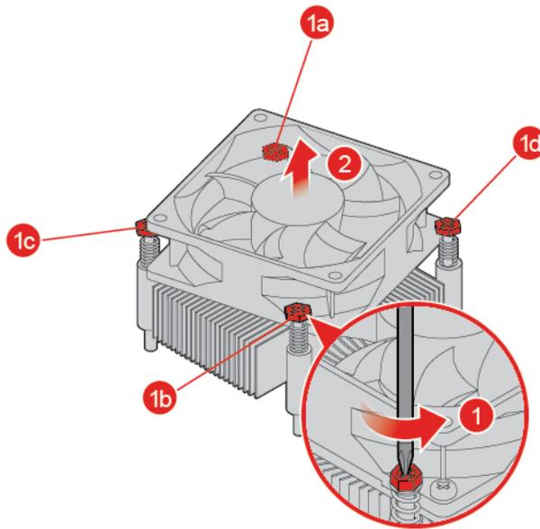
Figure 108. Removing the heat sink and fan assembly
