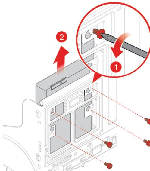
Figure 31. Removing the 3.5-inch primary storage drive
