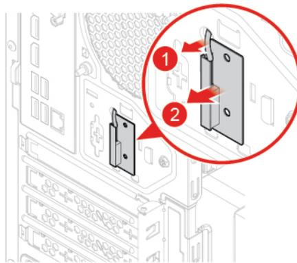
Figure 80. Removing the rear Wi-Fi antenna
