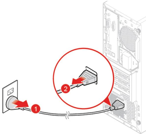
Figure 19. Removing the power cord
