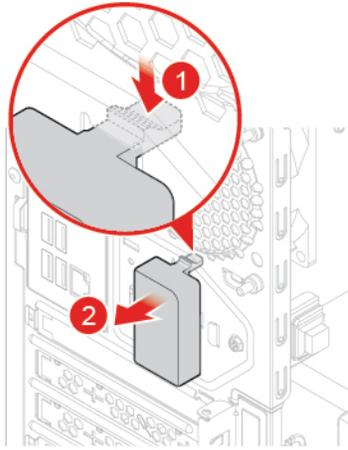
Figure 79. Removing the rear Wi-Fi antenna cover
