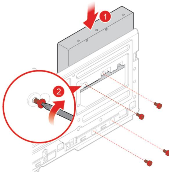
Figure 36. Installing the 3.5-inch secondary storage drive
