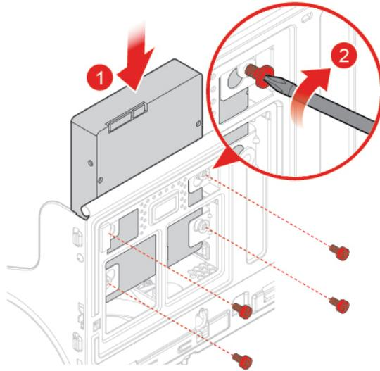
Figure 32. Installing the 3.5-inch primary storage drive
