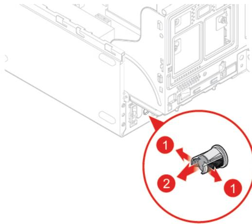
Figure 92. Removing the illuminated red dot cable
