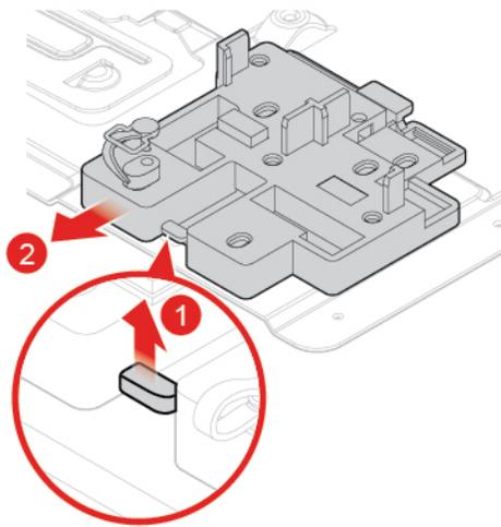
Figure 71. Removing the M.2 solid-state drive bracket
