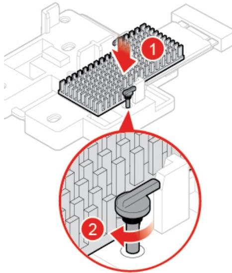
Figure 69. Installing the M.2 solid-state drive heat sink
