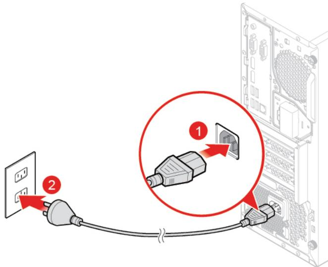
Figure 20. Installing the power cord
