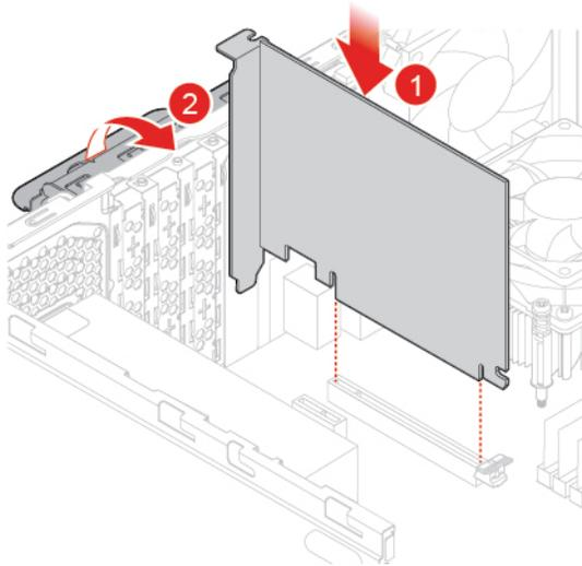
Figure 47. Installing the PCI Express card
