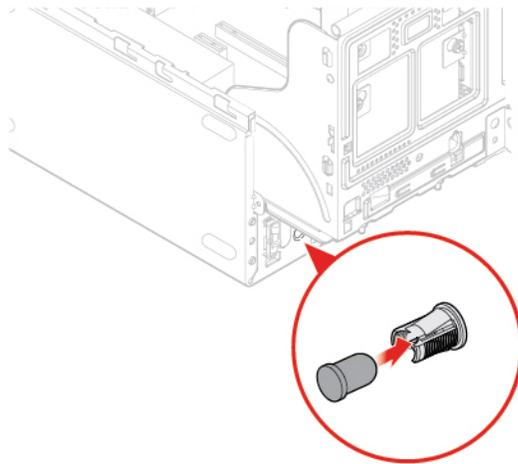
Figure 93. Installing the illuminated red dot cable
