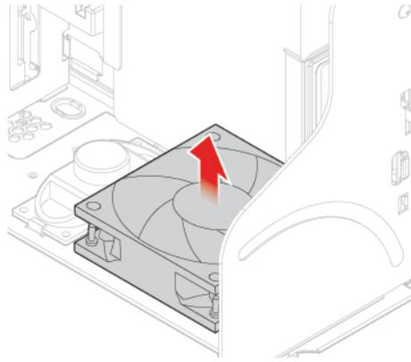
Figure 88. Removing the front fan
