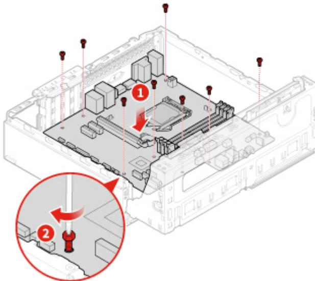
Figure 134. Installing the system board
