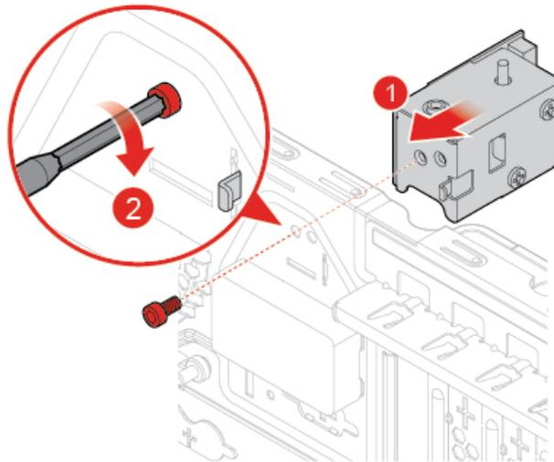
Figure 126. Installing the E-lock
