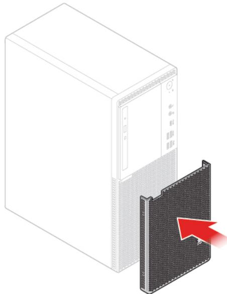
Figure 22. Installing the dust shield
