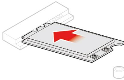
Figure 69. Installing the Wi-Fi card
