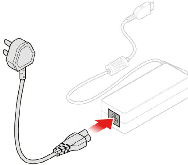
Figure 18. Installing the power cord
