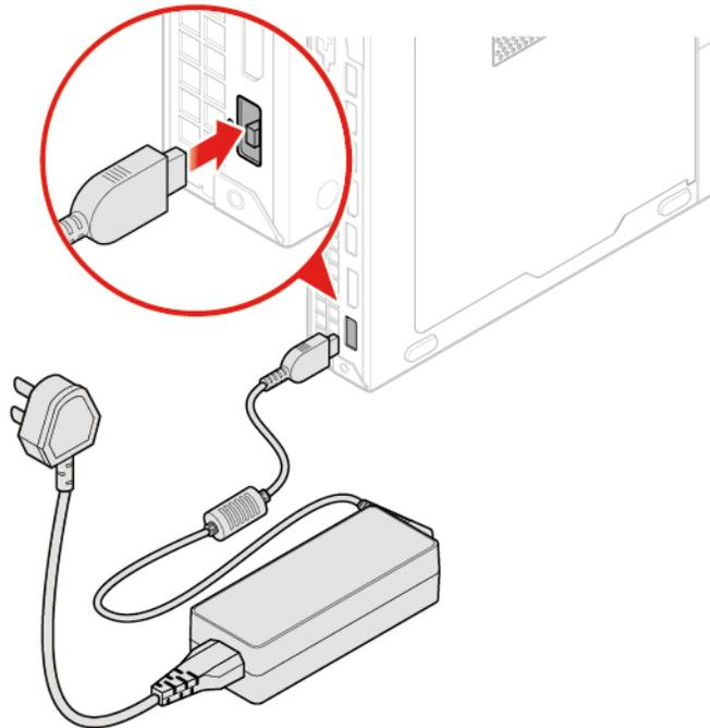
Figure 19. Installing the power adapter
