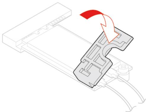
Figure 71. Installing the Wi-Fi card shield
