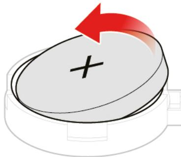
*Figure 51. Removing the coin-cell battery*
