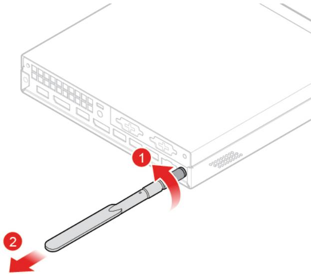
Figure 76. Removing the rear Wi-Fi antenna
