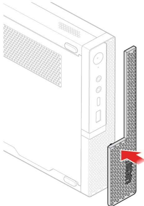
Figure 99. Reinstalling the dust shield
