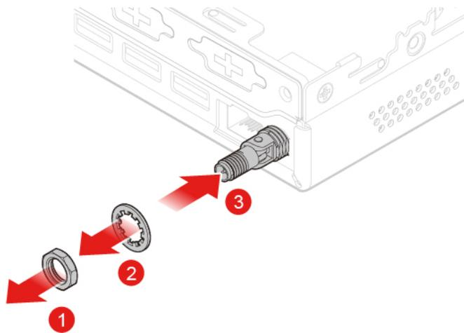
Figure 78. Removing the rear Wi-Fi antenna cable
