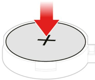
Figure 53. Pressing the coin-cell battery downward
