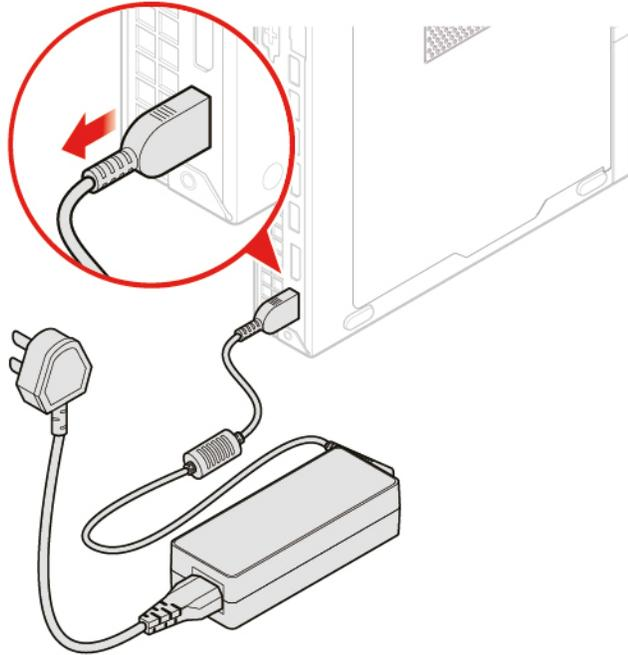
Figure 16. Removing the power adapter
