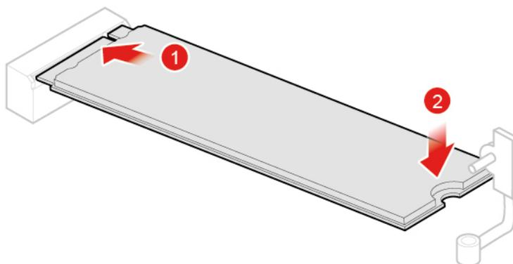
Figure 92. Installing the M.2 solid-state drive
