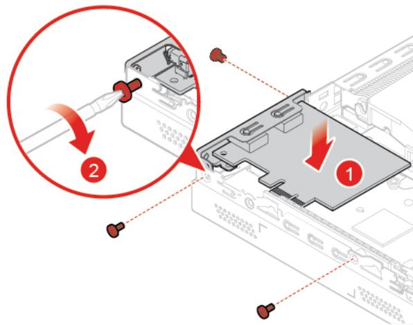
Figure 41. Installing the PCI Express card
