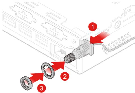
Figure 79. Installing the rear Wi-Fi antenna cable
