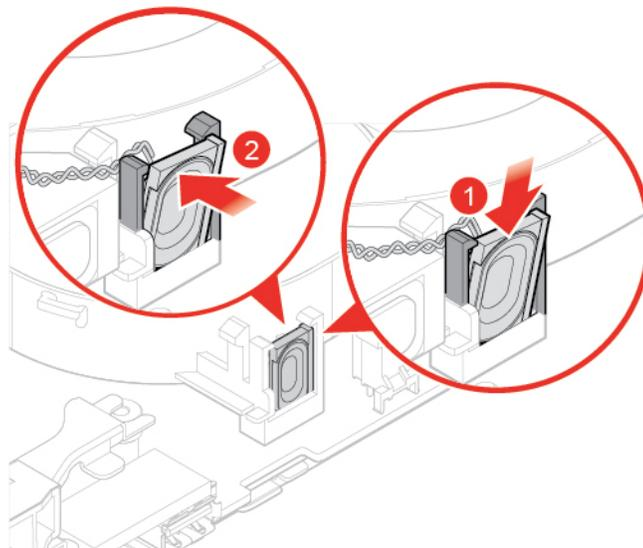
Figure 43. Installing the internal speaker
