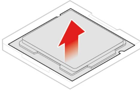
Figure 56. Removing the microprocessor
