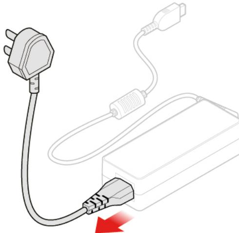
Figure 17. Removing the power cord
