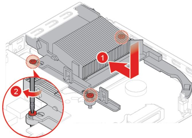
Figure 49. Installing the heat sink
