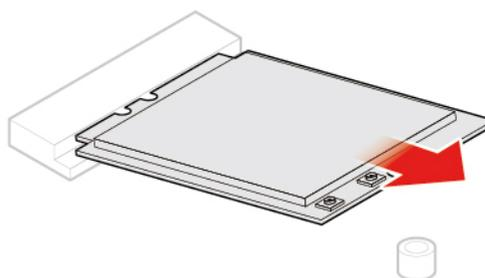
Figure 62. Removing the Wi-Fi card
