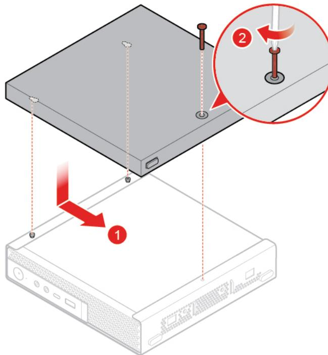
Figure 27. Installing the external optical drive box
