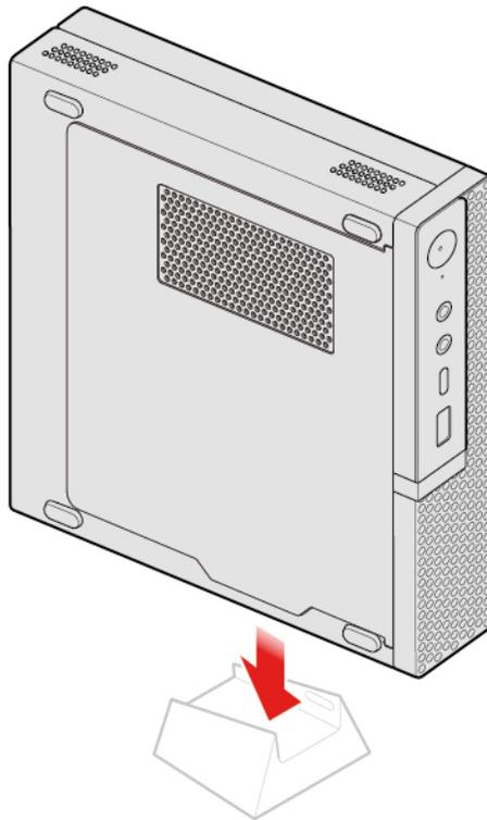
Figure 21. Installing the vertical stand
