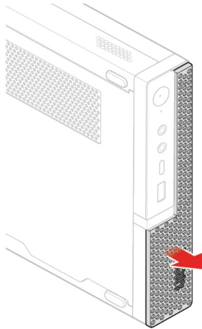
Figure 30. Removing the dust shield
