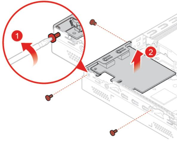
Figure 38. Removing the PCI Express card
