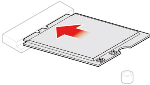
Figure 63. Installing the Wi-Fi card
