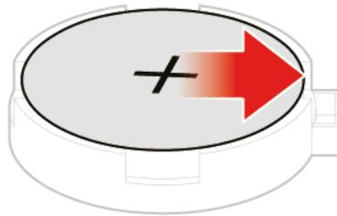
*Figure 50. Pressing the metallic tab*
