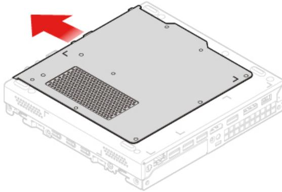
Figure 84. Removing the bottom cover
