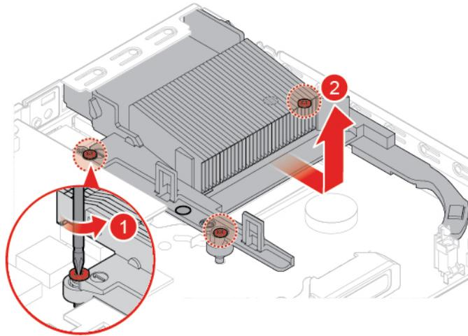
Figure 48. Removing the heat sink
