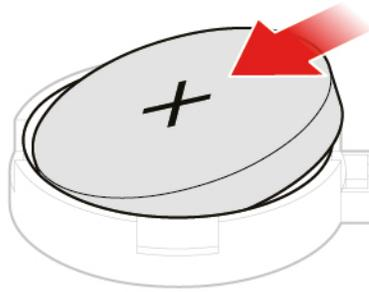
Figure 52. Installing the coin-cell battery
