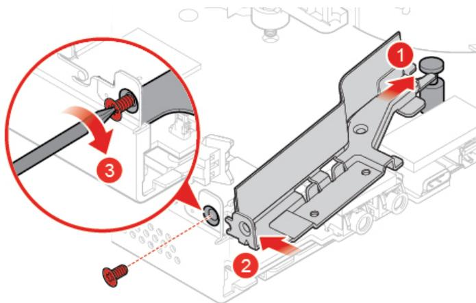
Figure 83. Installing the antenna bracket
