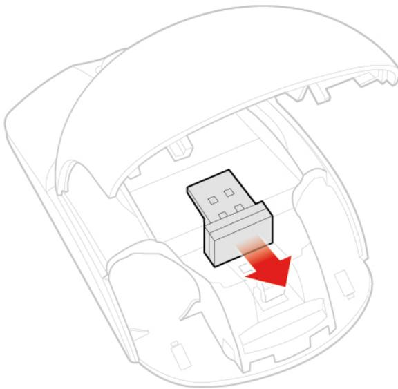
Figure 11. Taking out the USB dongle
