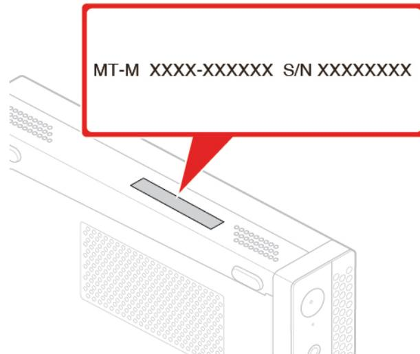
Figure 4. Machine type and model label
