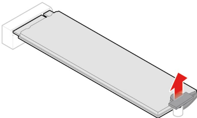
Figure 90. Unlocking the M.2 solid-state drive clip
