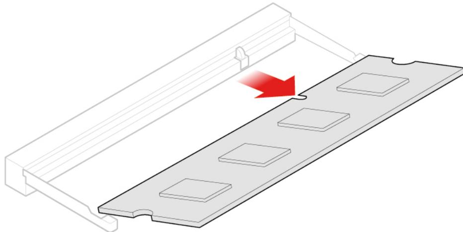
Figure 87. Removing the memory module
