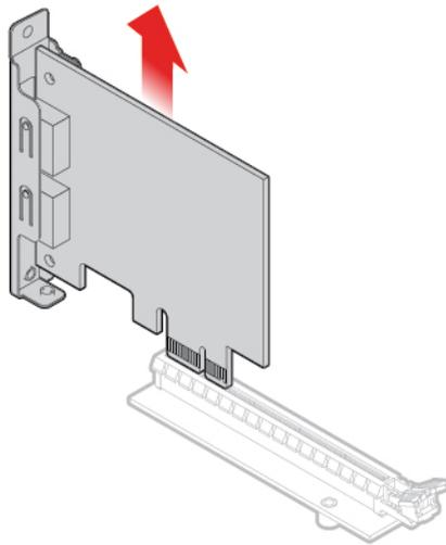
Figure 39. Removing the PCI Express card adapter
