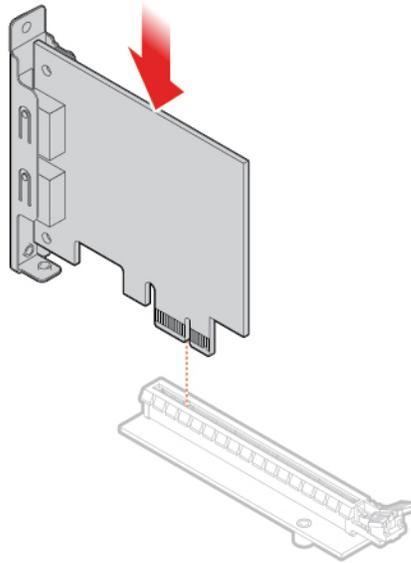
Figure 40. Installing the PCI Express card adapter
