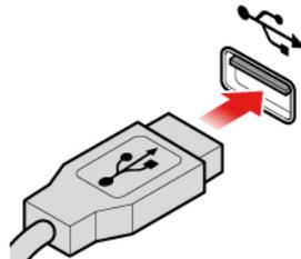
*Figure 7. Replacing the keyboard*
