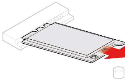
Figure 68. Removing the Wi-Fi card
