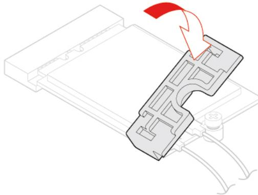
Figure 65. Installing the Wi-Fi card shield
