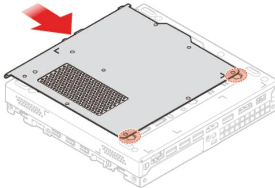
Figure 85. Installing the bottom cover
