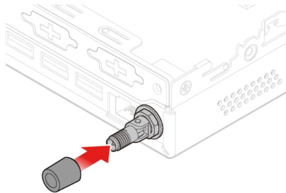
Figure 80. Installing the antenna cover to secure the rear Wi-Fi antenna cable
