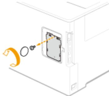
**2** Open the ROM cover, and remove it in the direction indicated by the arrow.
