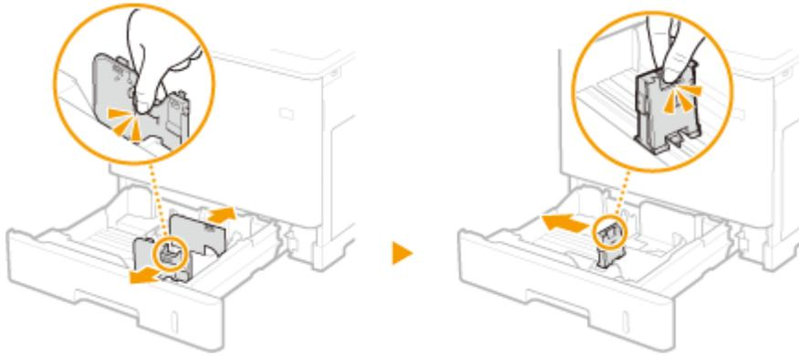
**3 Load the paper so that the edge of the paper stack is aligned against the right side of the paper drawer.**
