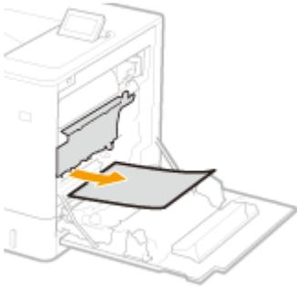
**3 Remove the jammed paper inside the duplex unit.**
