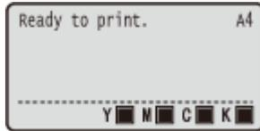
The display shows the printing status and the screens for specifying settings. It also shows error messages and the amount remaining in the toner cartridge.
