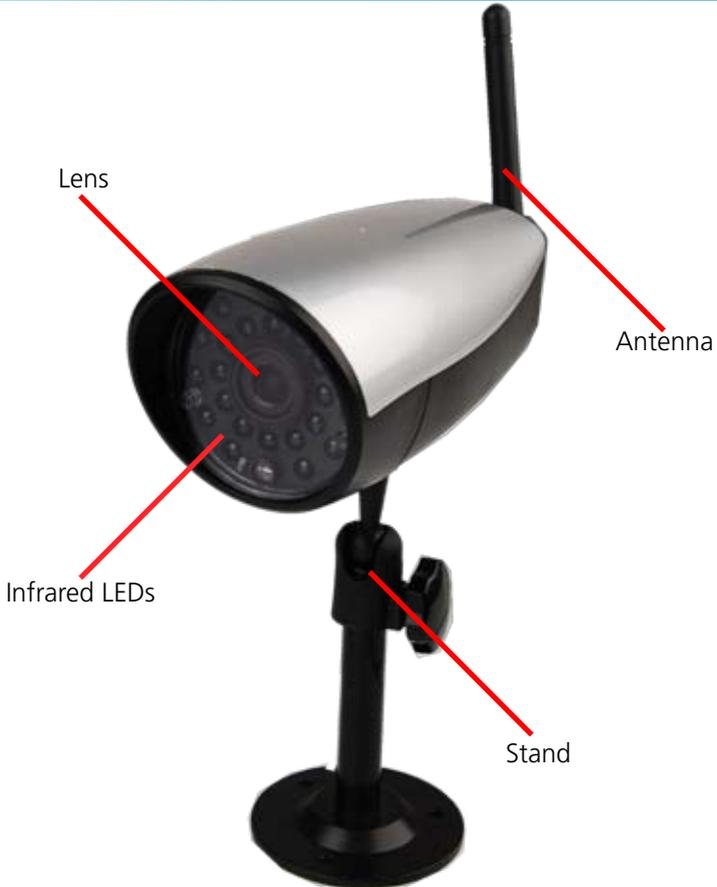
**Lens:** The business end of the camera. For a reliable and clear image, ensure that the lens stays clean and unobstructed. To clean, use a dedicated lens cleaning solution and cloth, available from all good photography stores.
