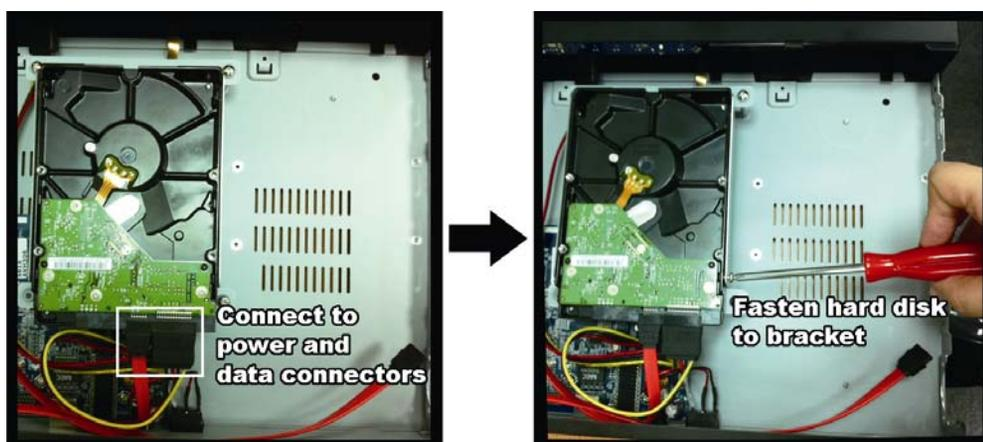
Step5: To install another hard disk, find the supplied hard disk brackets in the package, and fix them onto the NVR base.
