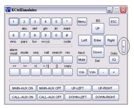
Please note that most of the buttons correspond to the keypads on the front panel. If you connect the PC through RS-232 and use an RS-232/RS-485 converter to connect to multiple DVRs, you would be able to control multiple DVRs via the simulation software. Please refer to <u>Section 3.2 Optional Connections</u> to connect/cascade the DVRs to the PC.
