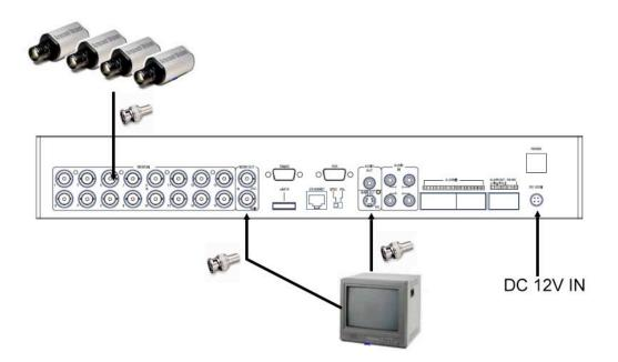
Please make sure to set the NTSC/PAL Selector Switch on the back panel according to the local TV system for the digital video/audio recorder to work correctly.
