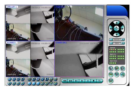
The video images can be displayed in several types of split-window screens, including 1/4/9/16-Window for single DVR and 25/36/49/64 for multiple DVRs. And the focus window is surrounded by a frame border. In addition to the video windows, there are different icons on the lower corner and the right corner of the screen for status display and control. (Please note that the ".L" following the
