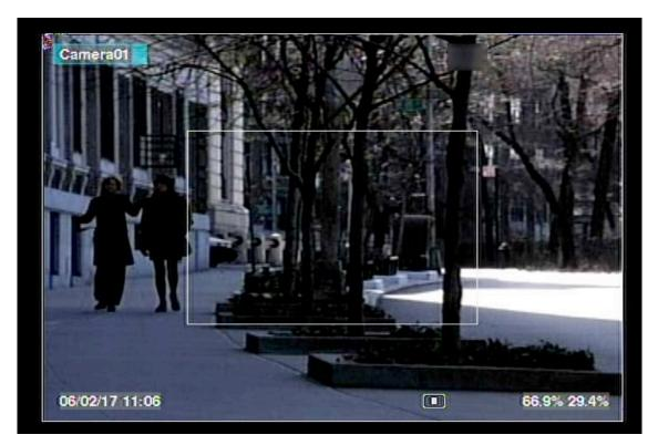
The system supports X2/X4 Digital Zoom function. To use this function, press X2 button (Mouse: ) in full screen display to enter Digital Zoom mode. There will
