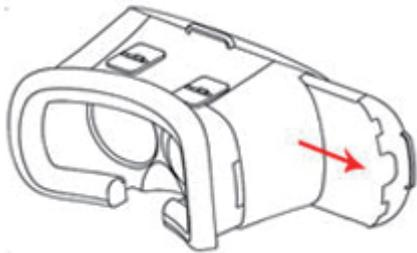
Insert your mobile phone into the holder on the front of the front section. The spring loaded holders will open and close to hold your phone securely.
