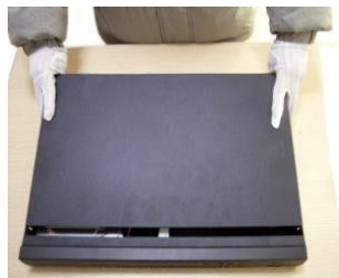
②disassemble the cover
