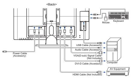
\* VGA (D-Sub) cable is not supplied with the monitor; you need to use a special VGA (D-Sub) cable dedicated for this model. Please contact the iiyama Support Centre in your country if you wish to connect the monitor via the VGA input.
