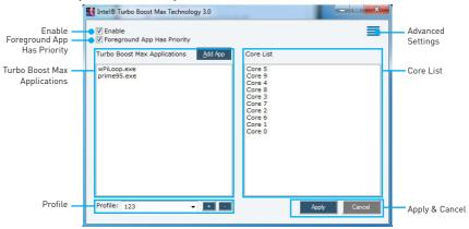
• Enable - allows you to enable Intel® Turbo Boost Max Technology 3.0 by checking the box. When the box is un-checked, the software returns the system to normal OS operation, which may not provide the best performance.
