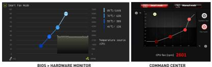
Both methods offer gradient points of the fan speed that allow you to adjust fan speed in relation to CPU temperature.
