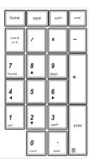
A numeric keypad is available on selected Notebook PC models. You can use this keypad for numeric input or as pointer direction keys.
