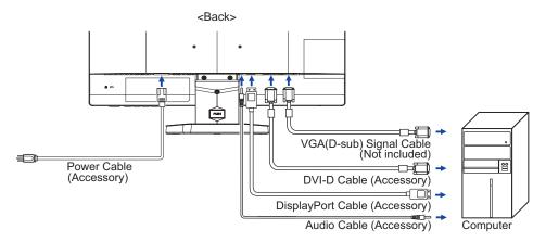
\* VGA (D-Sub) cable is not supplied with the monitor; you need to use a special VGA (D-Sub) cable dedicated for this model. Please contact the iiyama Support Centre in your country if you wish to connect the monitor via the VGA input.
