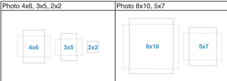
When QuickFit is activated, press the control buttons to make adjustments. The QuickFit OSD displayed in the lower right corner of the screen will guide users to make selections.
