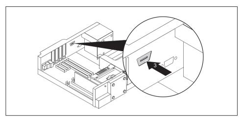
➤ To remove the break-out plate: carefully use a flat blade screwdriver to break out the plate (3). Dispose of the removed plate according to the national regulations.
