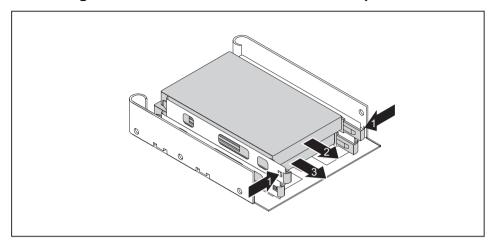
▶ Press the EasyChange rails on the drives slightly together (1) and pull the drives with the EasyChange rails one after the other out of the adapter (2, 3).
