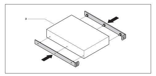
► Fasten the EasyChange rails to the side of the drive or adapter by inserting each pin of the EasyChange rail in the corresponding holes on the drive. In doing so, make sure that the ports on the drive are located at the rear as shown (a).
