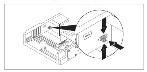
▶ To remove the spring metal cover: keep the clips (1) pressed and push the metal cover out of the casing from the inside (2).
