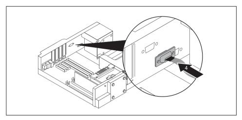
▶ Place the serial port inside the device at the position shown (see illustration, position 4).
