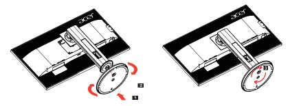
Remove: Reverse the steps to remove the base.
