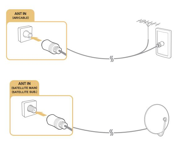
It is best to connect the both connectors using a Multi-Switch or DiSEqC. Switch, etc and to set **Aerial Connection Type** to **Dual Oscillator**.
