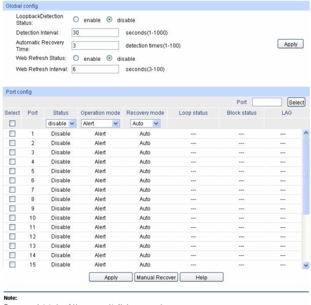
Recovery mode is just useful to process not in Alert process mode. LoopbackDetection must coordinate with storm control.
