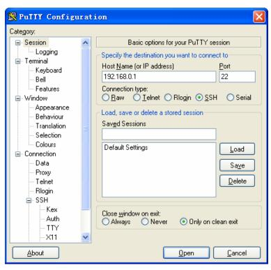
2. Click the **Open** button in the above figure to log on to the switch. Enter the login user name and password, and then you can continue to configure the switch.
