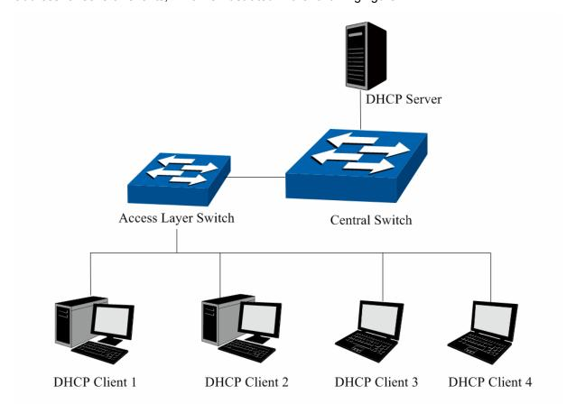
Figure 12-5 Network diagram for DHCP-snooping implementation
