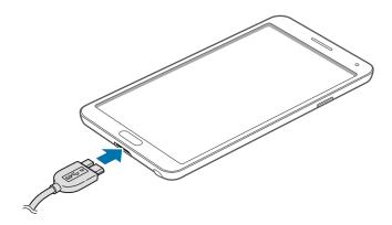
When using a USB 2.0 cable, plug the USB cable into the right side of the multipurpose jack as shown in the image below.
