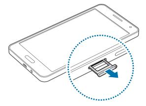
3 ► Dual SIM models: Place the SIM or USIM card on the SIM card tray with the gold-coloured contacts facing downwards.
