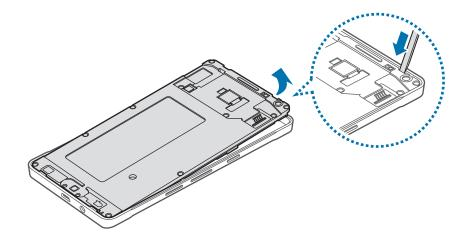
5 Disconnect the battery connector as shown in the image below.
