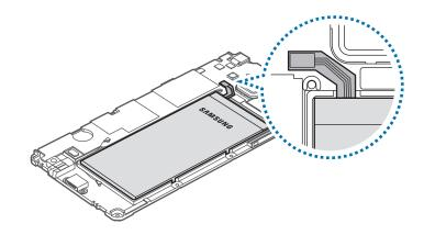
6 Push the back of the battery with your fingers and remove the battery.
