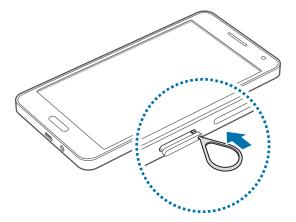
Ensure that the ejection pin is perpendicular to the hole. Otherwise, the device may be damaged.
