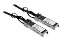
The SFPCMM1M Cisco Compatible 1m SFP+ cable is a fully hot pluggable, direct attach cable, supporting 10 Gigabit Ethernet and Fiber Channel applications connected through (Small Form Factor Pluggable) SFP+ ports.
